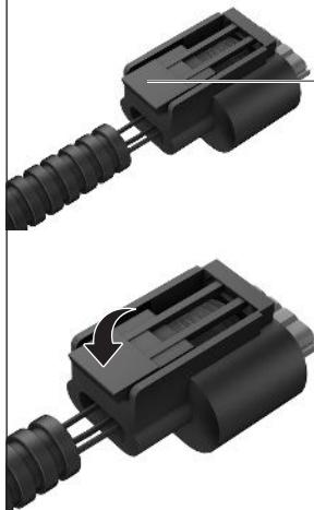
The plugs are locked into the connection sockets by means of a *locking clip*. Press the *locking clip* and pull the plug.
