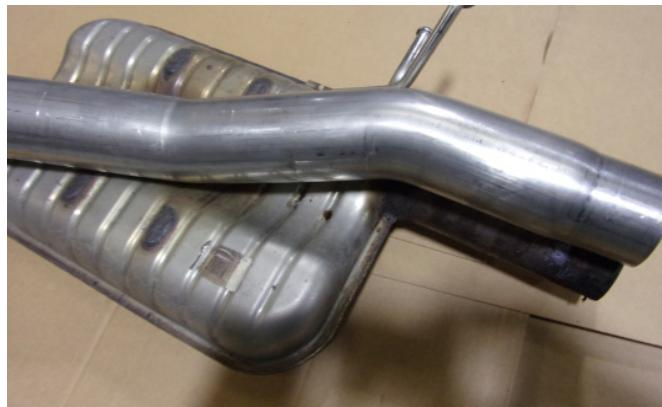
Remove the original system, place the resonator delete pipe over the top of the system.
