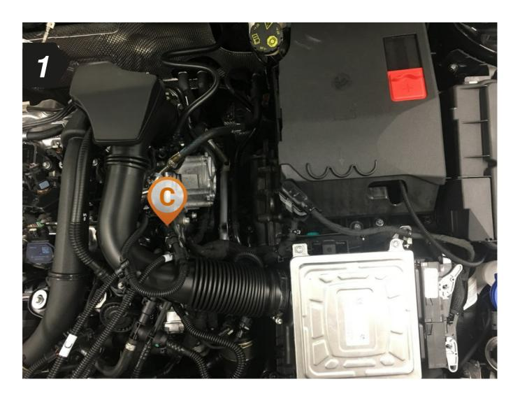
• To begin, locate the connection to the camshaft sensor in your engine bay.
