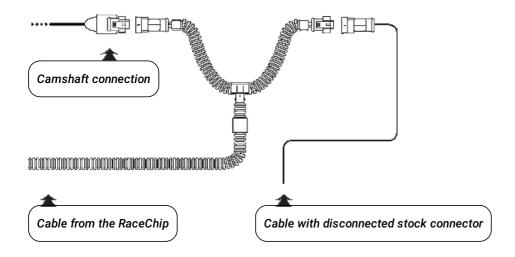
• Disconnect the plug from the camshaft sensor.
