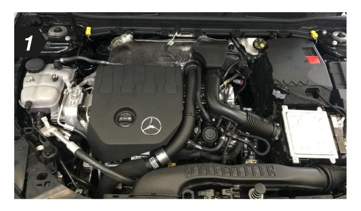
• Remove the engine cover and place it next to the car. You may have to jiggle the cover slightly to release it from the holding clips.
