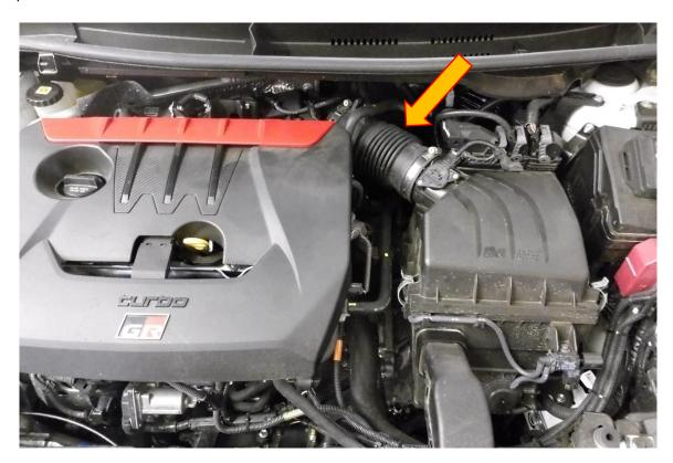
2. Using a 10mm socket and rachet loosen both hose clamps attaching the OEM turbo inlet hose. The oil breather hose can will simply pull off to remove from situ.
