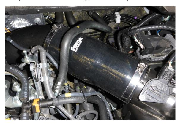
**14.** Re-route the vac hose which was originally attached to the OEM intake pipe. Use the supplied cable ties to secure it in place.
