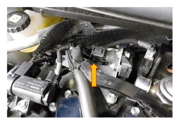
6. Using long nose plyers loosen the sprung hose clamp to allow you to remove the oil breather pipe.
