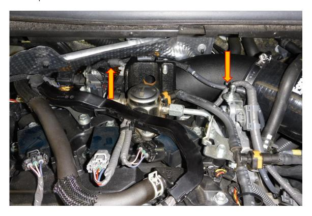
15. Please fully check your installation and ensure all fasteners are tight with no mis fit as a loose hose can activate the engines EML (Engine management light). Fit the engine cover to complete the installation of FMTIA8. Take your vehicle for a test and enjoy your new Forge Motorsport product.
