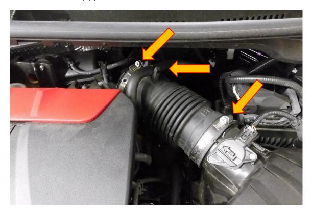
3. Detach the vacuum lines from the turbo inlet hard pipe clips shown by the arrowes below.
