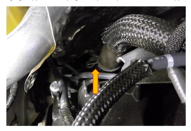
7. Remove the vacuum hose from the hard pipe, this will simply pull away to remove from situ.
