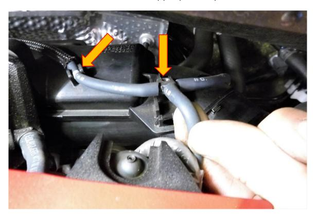
4. Using a 12mm socket and rachet remove both M8 fasteners attaching the inlet hard pipe to the engine.
