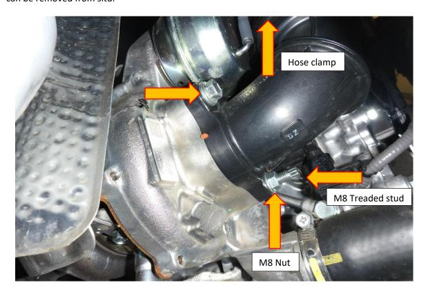
9. With the OE turbo adaptor removed pull the original red rubber O- ring out of its housing. Fit the O ring to the Machined coupler from the Forge kit. Using a 6mm Allen key and the supplied M8 cap head fasteners from the FMTIA8 kit, fit the Forge Motorsport machined billet adaptor to the turbo.
