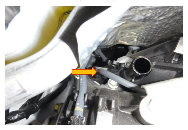
8. Using a 12mm socket and rachet or 12mm spanner remove the M8 fastener and M8 nut attaching the turbo elbow to the turbo. Using an E8 socket and rachet remove the threaded M8 stud from the turbo. Loosen the hose clamp at the other end of the turbo elbow, the turbo elbow can now be parted from the hard pipe and can be removed from situ.
