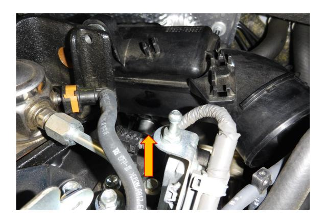
5. Using a 10mm socket and rachet remove the M6 fastener further down on the underside of the hard pipe.
