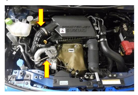
2. Pull out the engine oil dip stick and using some long nose pliers or hose removal tool loosen the hose clamp attaching the oil breather and remove the hose from the engine.
