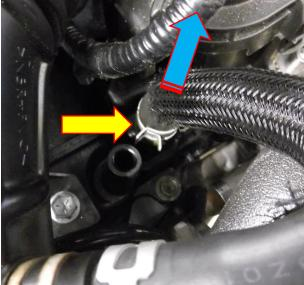
3. Fit the Forge silicone hose in replacement of the original turbo inlet hose. Using a 7mm socket and ratchet secure the hose using the supplied hose clamps. 40-60 clamp will secure the turbo end of the hose and the 60-80 hose clamp will secure the airbox end of the hose.
