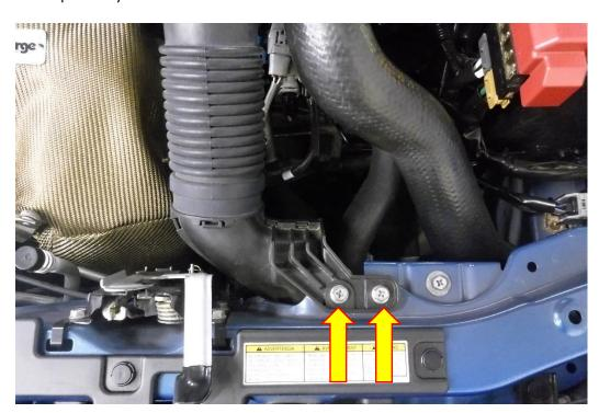
4. Pull the vacuum pipe attached to the airbox to disconnect it. Using a 10mm socket and rachet remove the X2 M6 fasteners attaching the airbox to the engine. The airbox will now lift out of its mounting points.
