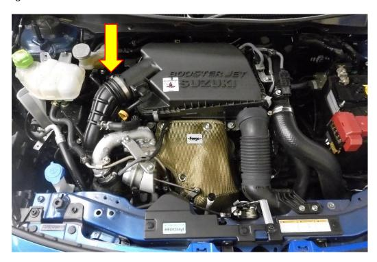
2. Unplug the MAF sensor by depressing the tab, then using a pozi drive screwdriver remove the two fasteners attaching the sensor to the airbox. The MAF sensor will now remove from the airbox.
