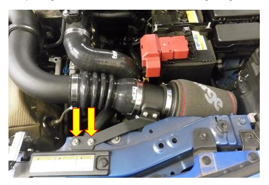
17. Adjust the silicone hose and filter if needed to the preferred orientation the using a 7mm socket and ratchet, now tighten all 3X hose clamps.
