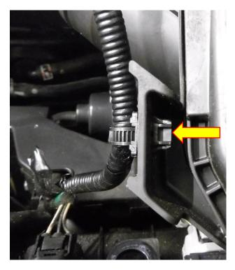
6. Using an 8mm socket and ratchet loosen X2 hose clamps securing the boost hose. The hose can now be removed from situ.
