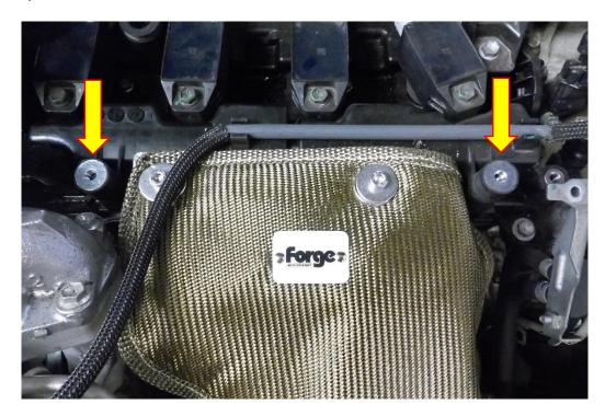
8. Using a 5mm Allen key attach the supplied M6x8 button head fastener, M6 washer and alloy mounting peg to the mounting plate in the same location as shown in the picture below.
