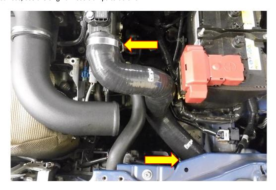
14. Using a 5mm Allen key attach the mounting bracket to the small hard pipe using the supplied 2X M6x8 fasteners and M6 spring washers. Attach the filter from the FMINDK53 kit to the hard pipe as shown in the picture below, but do not tighten the hose clamp at this stage.
