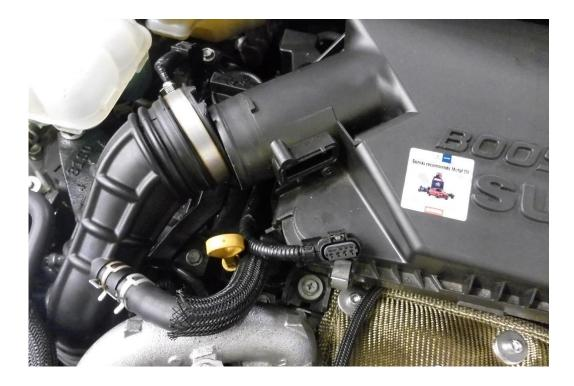
3. Using a 10mm socket and ratchet remove the X2 M6 fasteners attaching the air duct to the slam panel, the duct will now pull away from the air box.
