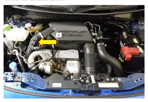
2. Using an 8mm socket and suitable drive or flat blade screwdriver loosen both hose clamps attaching the turbo inlet hose. Use plyers to loosen the hose clamp attaching the breather hose and disconnect it from the turbo inlet hose. You will now be able to remove the turbo inlet hose from the vehicle.
