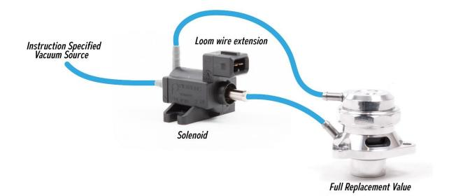
14. Plug the supplied wiring loom to the vehicle DV plug and the other end to the solenoid.
