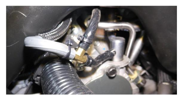
9. Run the remaining vacuum hose along the back of the engine to the coolant tank, securing it to the bulkhead using the supplied cable ties at the points shown by the large arrows in the below images.
