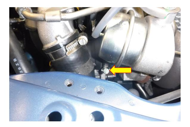
3. Locate the original DV attached to the turbo, slide back the locking tab on the DV plug then press in the retaining clip to disconnect the wiring loom to the DV.
