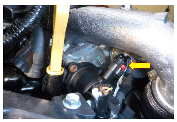
4. Using a T30 Torx and suitable drive remove the X3 fasteners attaching the original DV to the turbo.
