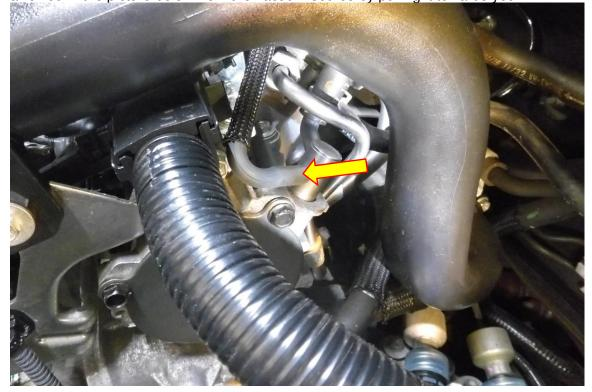
8. Using some side cutters cut a small length of the supplied vacuum hose to size and fit the vacuum T piece as shown in the picture below. Secure the hoses with the supplied small cable ties.
