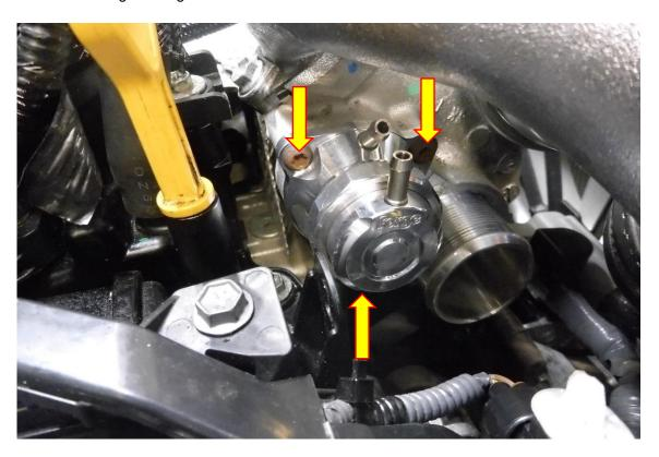
7. Locate the vacuum source which is at the back right of the engine. Disconnect the hose arrowed in the picture below from the vacuum source by pulling it towards you.
