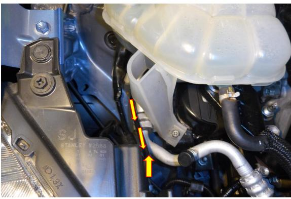
10. Using a 10mm socket, extension and suitable drive remove the M6 fastener attaching the lower coolant tank bracket.
