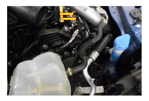
16. Re-fit the turbo elbow and oil breather to complete the installation of FMDV47. Take the vehicle for a test drive and enjoy your new Forge Motorsport product.
