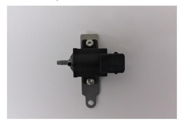
12. Mount the solenoid bracket to the lower coolant tank bracket in the orientation shown below. Using a 10mm socket and suitable drive attach the supplied M6 fastener and penny washer to secure both.
