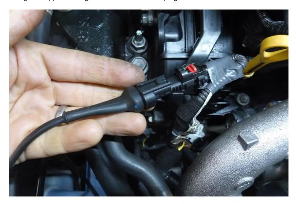
15. Using side cutters cut the vacuum hose to length and use the supplied cable ties to secure in place. Bunch up the vacuum hose and the wiring loom using the larger cable ties to neaten the install.
