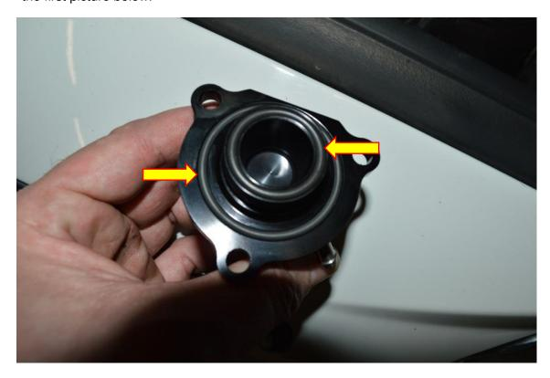
6. Mount the Forge Motorsport valve to the turbo in the same orientation as the picture and secure it using the original x3 fasteners with a T30 Torx and suitable drive.
