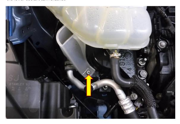
11. Using a 3mm Allen key and the supplied 2x M4 fasteners attach the solenoid to the bracket as shown in the picture below.
