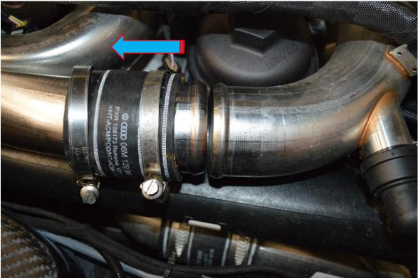
4. Using a 32mm socket and suitable extension remove the oil filter housing by turning in an anticlockwise direction. We would recommend covering the void with a latex glove or similar to stop debris or deposits entering the exposed aperture.
