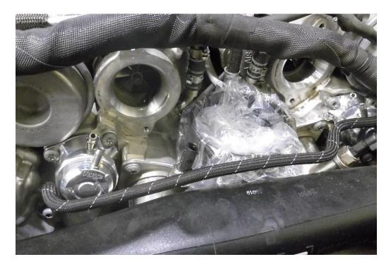
11. Starting with the left-hand side valve, connect one of the wiring looms supplied with the FMDV27 kit to the OE valve wiring loom. Run the loom under the oil breather and connect one of the solenoids from the FMDV27 kit.
