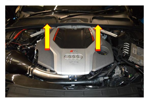
2. Using a trim tool remover or flat bladed screwdriver pry the clips that hold the wiring loom away from the inlet tracts as arrowed below.
