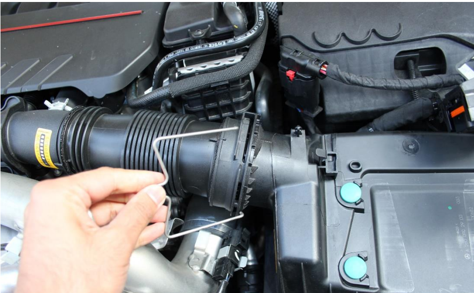
7. Remove the spring clip from the tube connection.
