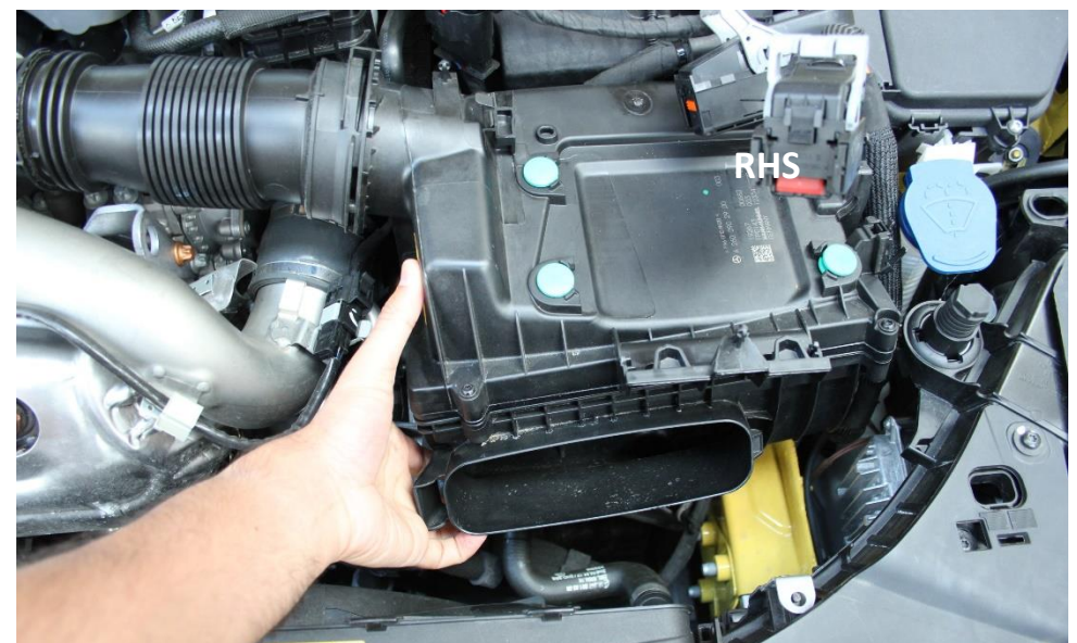
8. Pull the airbox upwards from the front.
