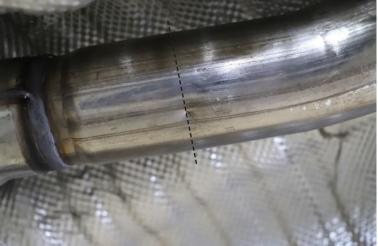
To make it easier to cut the exhaust we recommend removing it from the car. Find the indent just before the resonator to mark out the cutting line. Cut along the line and de-bur the edges. If fitting with the original GPF-back re-fit this now and then fit the Scorpion GPF delete following the line diagram on the first page. If fitting with the Scorpion GPF-back you do not need to use the supplied adaptor.
