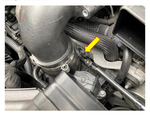
4. Remove the hose from the engine bay by pulling the throttle body end out first.
