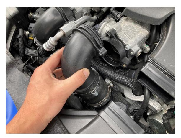
5. Remove the X2 M6 fasteners using a 5mm Allen Key, which attaches the throttle body adaptor to the throttle body. The adaptor will now pull away from the throttle body.
