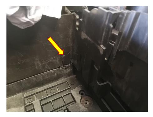
9. Using a flat blade screwdriver depress the tab arrowed in the image below and remove the fuse holder from situ.
