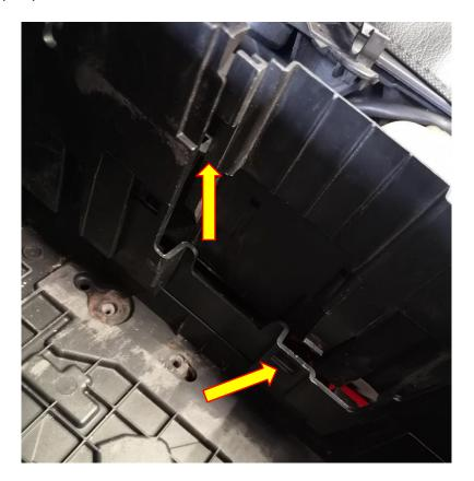
**7.** Using a 10mm socket and suitable drive remove the fastener on the left side of the battery tray.
