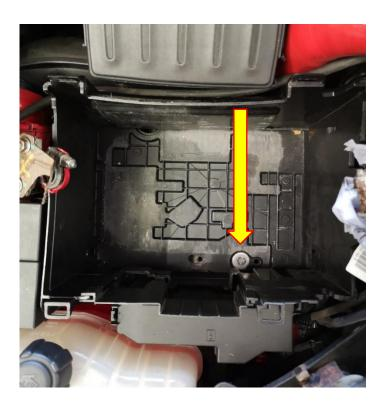
6. To remove the upper half of the battery tray, depress the two tabs on the right side of the battery tray.
