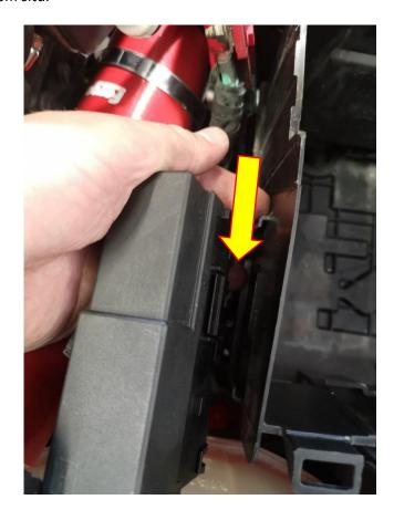
**10**. Slide the fuse box at the front of the battery tray upwards so that it disconnects from the battery tray.
