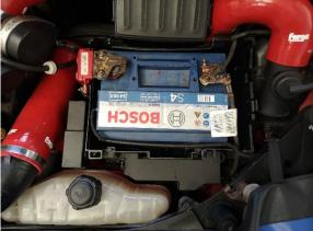
4. Using a 10mm socket and suitable drive disconnect the battery terminals undoing the **NEGATIVE TERMINAL FIRST**. Using a 13mm socket, extension and suitable drive undo the fastener at the front of the battery, this clamps it down into place. You can now remove the battery from the vehicle.
