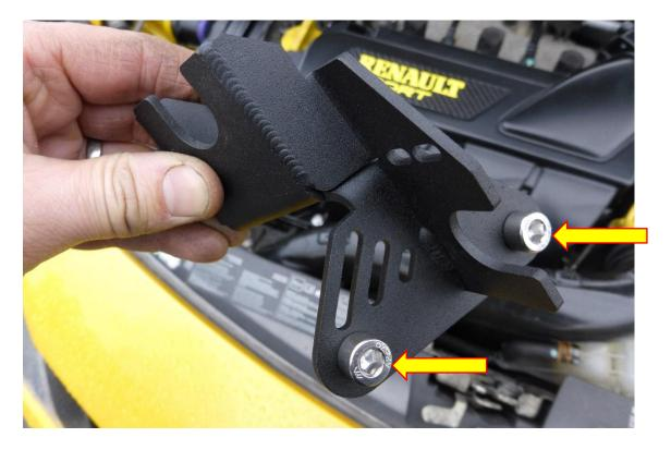
**21**. Take the X2 M4 fasteners and screw them into the cable bracket as shown in the picture, then push fit the top gear selector cable into position. This is the same for both cables.
