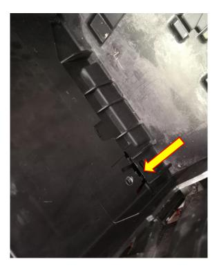
8. Depress the tab at the back left of the battery tray.
