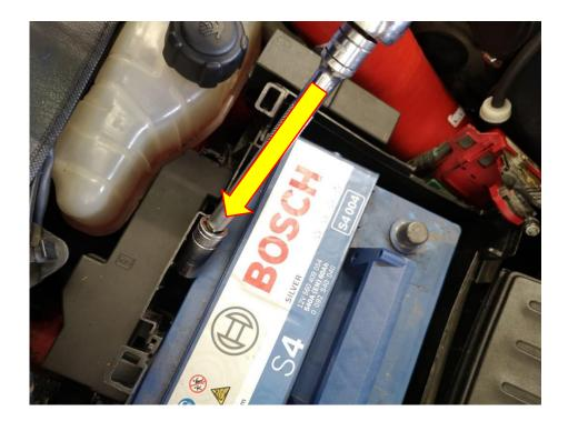
5. Using a 10mm socket and suitable drive remove the fastener at the front of the battery tray.
