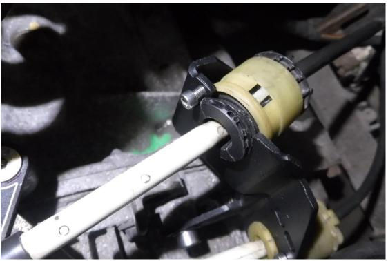
Using a 3mm Allen key tighten both fasteners to secure the side gear selector cables in the bracket.
