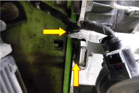
13. Using a T27 Torx driver remove both fasteners on each side of the crash bar.
