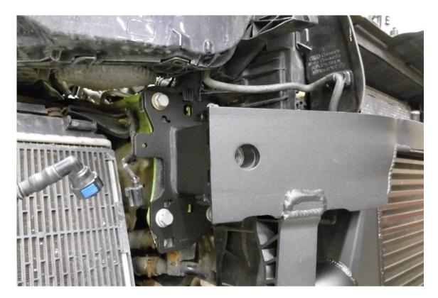
25. Using a 6mm Allen key secure the supplied temp sensor bracket using the supplied M6 fastener and washer, then install the temperature sensor to the bracket removed in step 11.
