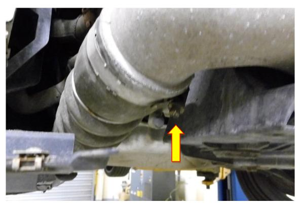
18. Using a T27 Torx driver remove the X4 fasteners (x2 each side) attaching the intercooler to the vehicle.
