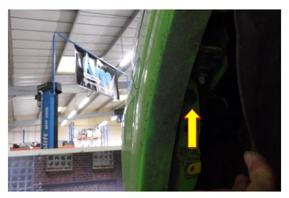
7. Feeling inside the wheel arch, underneath the liner you will be able to feel the clip for the bottom of the outer wheel arch trim. Squeeze this together as you gently pull on the bottom of the trim to release it and then work your way around until you have enough removed that the corners of the bumper will be free to come out.
