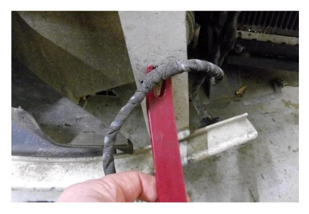
12. Unplug the horns by depressing the tab arrowed in yellow, then unclip the wiring loom connected to the crash bar. Using a T27 Torx driver remove the fasteners attaching the horns to the crash bar.
