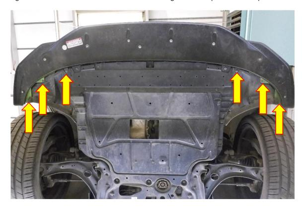
10. Pull both sides of the bumper away and release it from the vehicle, but not fully. Unplug the parking sensor loom and disconnect the headlight washers by depressing the retaining clip and pulling the pipe upwards and empty the washer fluid into a suitable container.
