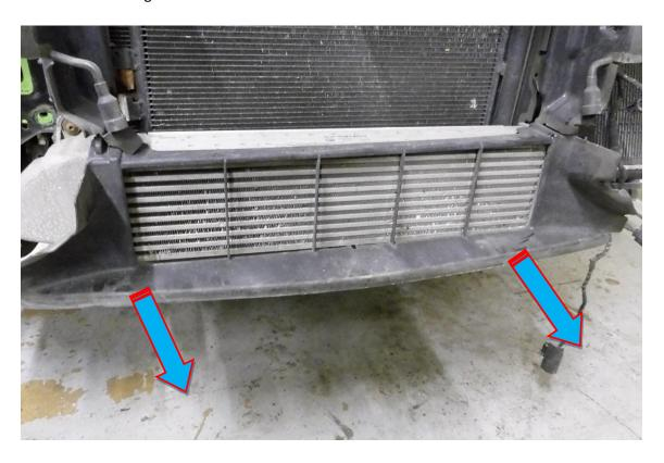
**16.** Pull the radiator airduct away from the vehicle, unclip the tubing for the headlight adjusters.
