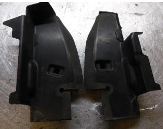
22. Reinstall the modified air ducting to the vehicle on both sides and refit the head light adjusters also.
