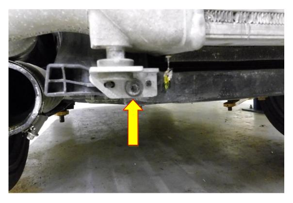
19. Install the rubber mounting grommets and alloy inserts into the intercooler as shown in the pictures.
