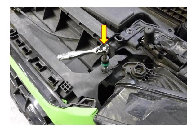
5. Using a T25 Torx driver remove the 3 X fasteners attaching the inner wheel arch liner to the vehicle on both sides.
