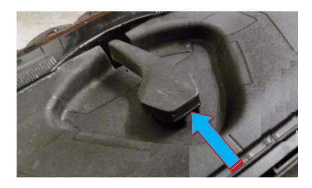
3. Remove the plastic slam panel by pulling it upwards from the edge.
