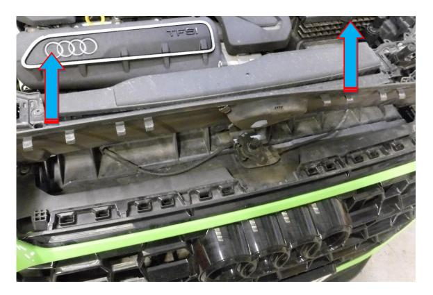
4. Using a T25 Torx drive remove the 2X fasteners (one each side) attaching the top of the bumper to the vehicle.
