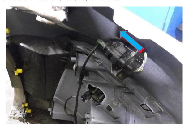
12. Un-plug both sides of the crash bar foam, then remove the foam from the crash bar completely. IMPORTANT: Depress the red locking clip on the plugs back first to allow removal!
