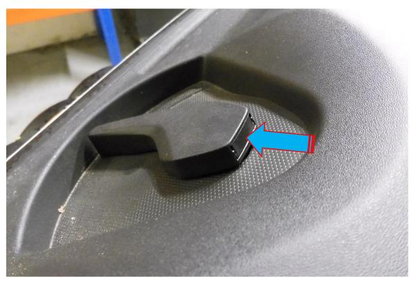
2. Using a trim removal tool prise the corner of the slam panel cover to allow your hand to get underneath it, then pull the front section upwards to release all the mounting clips. Now pull the cover towards you to remove it completely.
