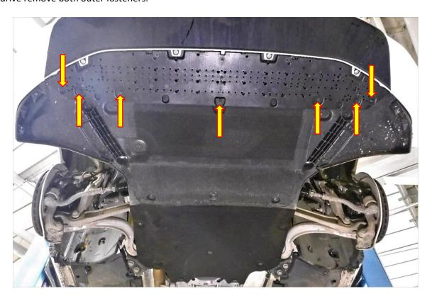
10. You will now be able to pull the sides of the bumper away from the wings and then the whole bumper will come away from the vehicle. IMPORTANT: do not pull the bumper fully from the vehicle till step 11 has been completed!
