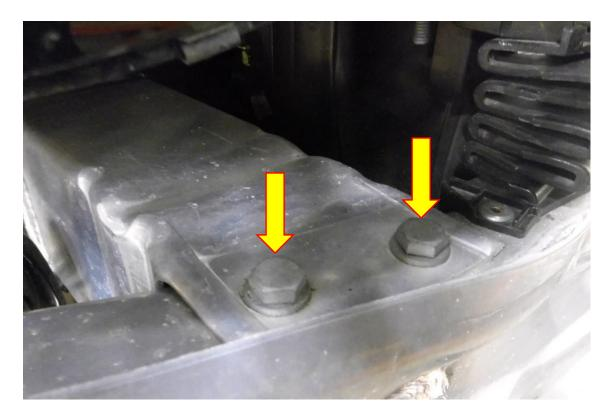
15. Using a T30 Torx driver remove X2 fasteners attaching the middle of the crash bar to the vehicle.
