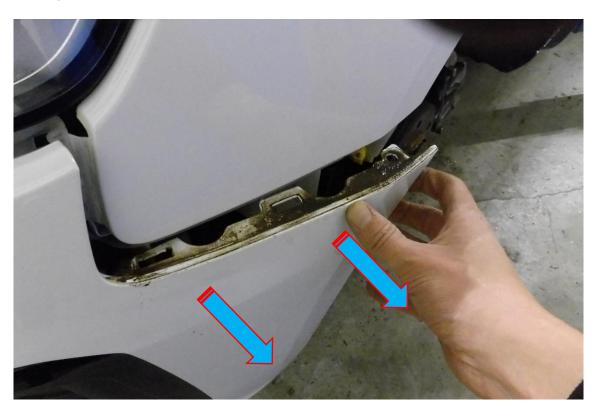
11. Depress the tab on the connecting plug and disconnect the parking sensor loom from the bumper, you will now be able to remove the bumper completely from the vehicle.
