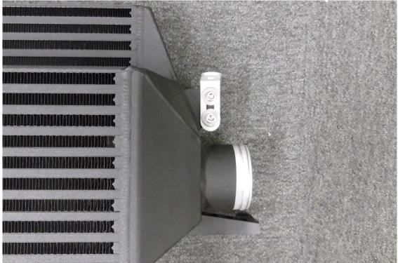
20. Place the intercooler into position, the lower mounting pegs on FMINT26 locate in the same position as the OE intercooler. Now replace the crash bar back into position.
