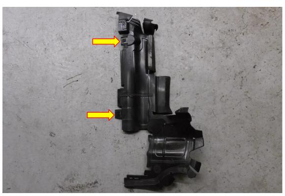
18. Using some long nose plyers press in both locking tabs at the top of the intercooler, you will now be able to pull the intercooler from the vehicle.
