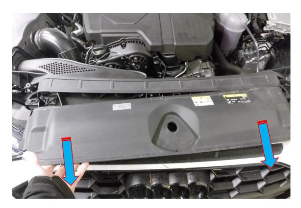
3. Using a T30 Torx drive remove the X4 fasteners attaching the top of the bumper to the vehicle.
