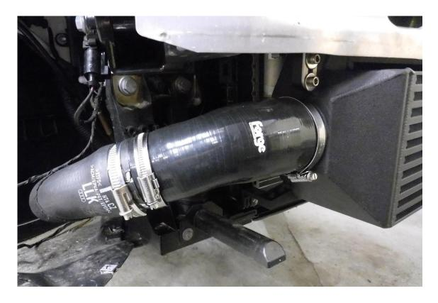
23. Take the remaining hose joiner, hose **#2052** and hose clamps and install them in the same way to the other side of the intercooler.
