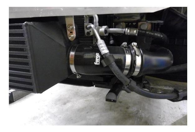
24. Using a drill with a 4mm drill bit make a hole in the temperature sensor braket and crash bar. Now using a T25 torx drive attach the temperature sensor to the crash bar with the supplied Torx fastener.
