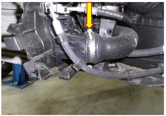
17. Using a flat blade screwdriver or trim tool press in the locking tabs for the intercooler ducting X2 on each side, then pull the ducting from the vehicle. **IMPORTANT: Do not re-fit ducting.**
