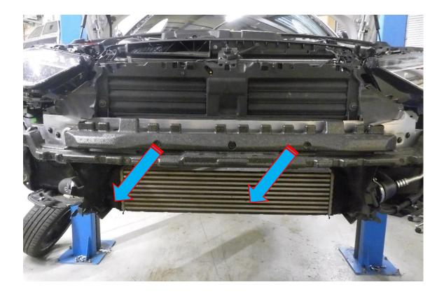
. Un-plug the temperature sensor loom and using a flat bladed screwdriver or trim tool remove the temperature sensor and bracket from the crash bar.
