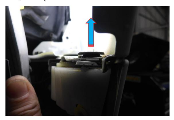
9. Looking from underneath the vehicle use a T30 Torx drive to remove 5X fasteners then using a T25 Torx drive remove both outer fasteners.
