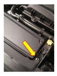
2. Unclip the coolant hose from the front airbox panel.
