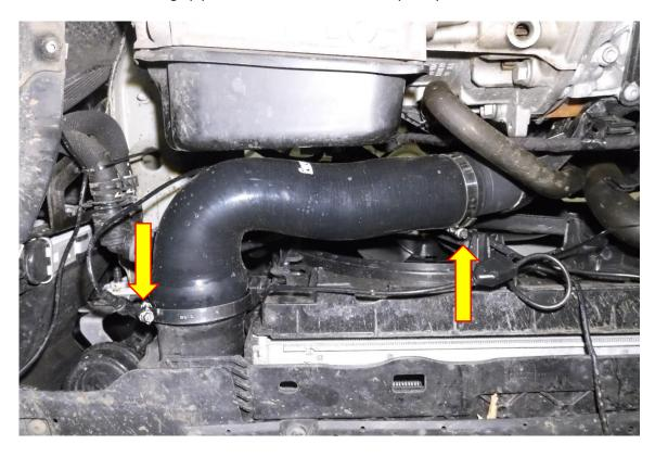
16. Looking from above disconnect the wiring harness attached to the OE discharge pipe and from the plastic loom clamp, you will now be able to wriggle the OE discharge free from the engine bay.
