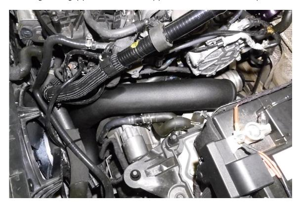
20. Take Hose #2055 from the FMDP1 kit and fit the large end to the Forge discharge pipe and the smaller end to the turbo. Do not tighten the hose clamps at this stage, the hose clamp 50-70mm is to be used at the smaller end and 60-80mm hose clamp to the larger end of the hose.
