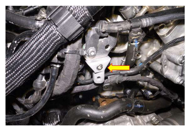
18. Using long nose plyers or hose clamp removal tool adjust the hose clamp on the heat exchange on top of the gear box, move the release side of the hose clamp clockwise to the side to avoid it making contact with the Forge discharge pipe.
