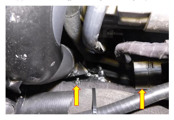
17. Using a 5mm Allen key attach the machined bracket and M6 fastener from the FMDP1 kit to the same mounting point from step 10.
