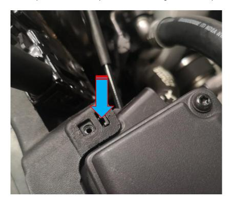
7. Pull sharply on the engine cover upwards to remove from situ.
