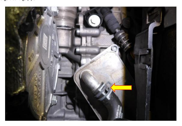
19. Place the Forge discharge pipe in situ where the OE pipe was removed as shown in the picture below.
