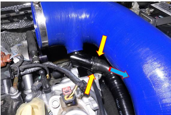
9. Using a 7mm socket and rachet or suitable flat blade screwdriver loosen both hose clamps attaching the OE discharge hose as arrowed below, now remove the hose completely.
