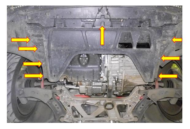
13. Looking from underneath the vehicle and using a T30 Torx driver remove the remaining fastener attaching the OE discharge pipe to the bottom of the engine.
