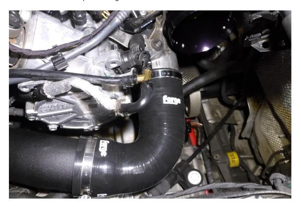
${\bf 21.} \ Using the supplied cable tie secure the coolant hose to the wiring loom behind it.$
