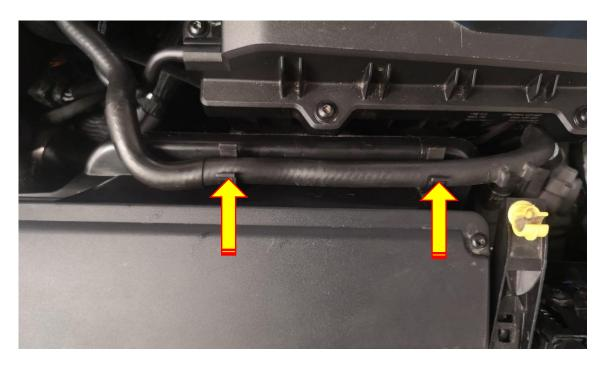
3. Using either a hose clamp removal tool or 7mm socket and suitable drive, disconnect the OEM or Forge inlet hose.
