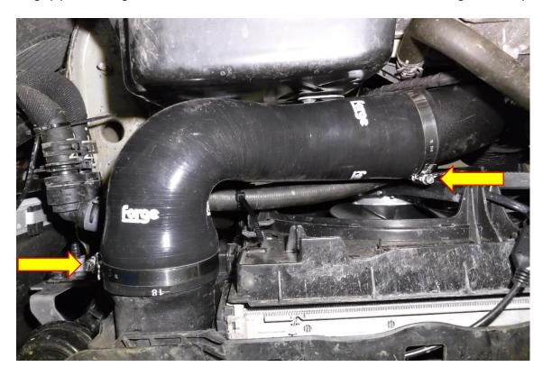
23. Re- attach the coolant hose to the hose clamp.
