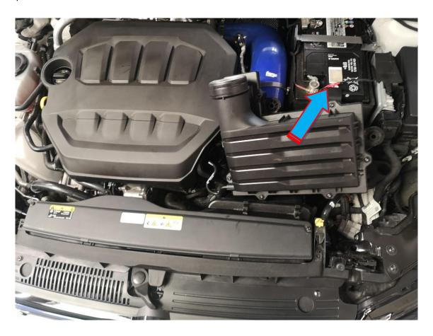
6. Press the tabs down and pull the front airbox panel towards the engine and then upwards to remove it.
