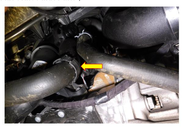
24. Take the P clip from the FMDP1 kit and place it round the Forge discharge pipe. Using a 5mm Allen key secure the P-clip to the machined adaptor fitted in step 17 using the remaining M6 fastener from the kit. Using a 7mm socket and ratchet or flat blade screw driver tighten the hose clamps the silicone joiners to the enlarged discharge pipe and all junctions.
