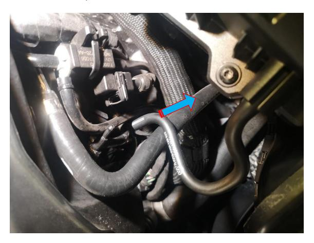
5. The airbox is located by rubber grommets on three pins. Rock the airbox left to right while pulling sharply in an upwards motion to remove it from situ.
