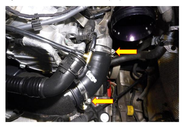
10. Using a T30 Torx driver remove the fastener attaching the OE discharge pipe to the engine.
