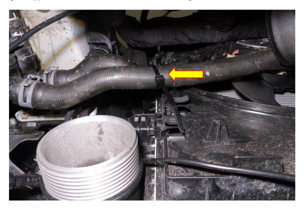
22. Depending on which option you have purchased, fit hose FMDP1 or FMDP3 to the intercooler and Forge discharge pipe and using a 7mm socket and ratchet secure the hose with the remaining hose clamps.
