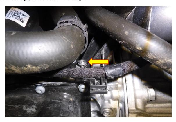
14. Unclip the water hose from its locating clamp and position the wiring loom the other side of the mounting bracket. Easiest way is to cut the tape with a sharp knife. (TAKE CARE NOT TO DAMAGE THE WIRING LOOM)
