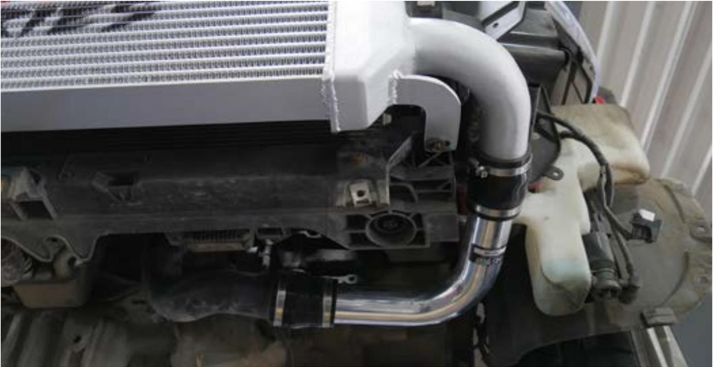
9. On the other side, now also mount the supplied silicone hoses and the aluminum tube with the charge air cooler and the original pressure pipe.
