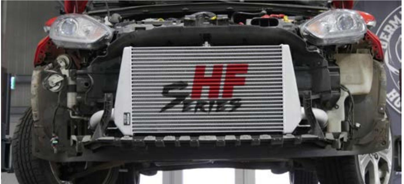
11. Depending on the gap dimension of the vehicle, it may be necessary in individual cases to adjust the bumper in the marked area with workshop tools on the inside in the direction of the charge air cooler.
