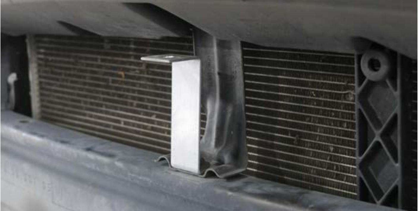
7. Mount the charge air cooler at the original holding points at the bottom, and with the screw supplied, at the top of the previously mounted bracket.
