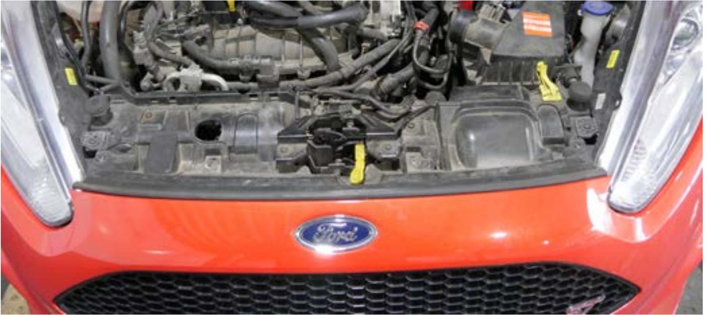
3. Remove the lower bumper bracket with the 10mm plug-on attachment
