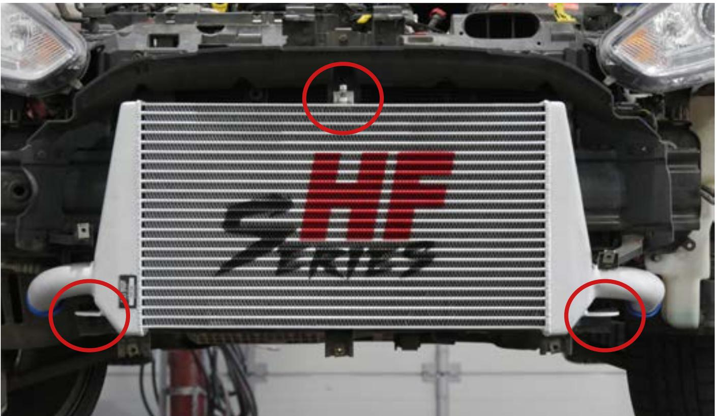
(Depending on the design, it may be necessary to bend the upper bracket slightly towards the bumper)
