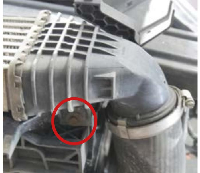
5. Pull the loosened cooler forward with a downward movement.
