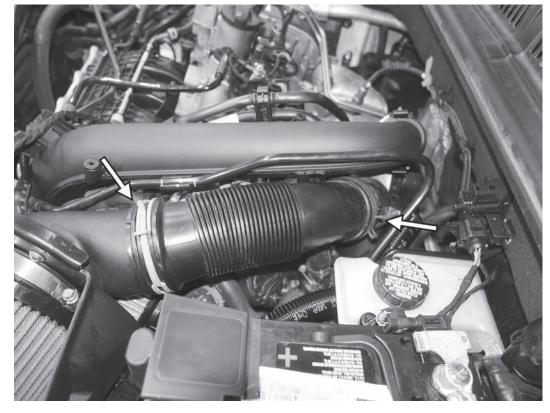
13) Install the accordian tube, connecting it to the APR airbox outlet and to the inlet of the turbo. Squeeze each of the spring clamps and slide them into their original positions to secure the accordian tube to the engine.
