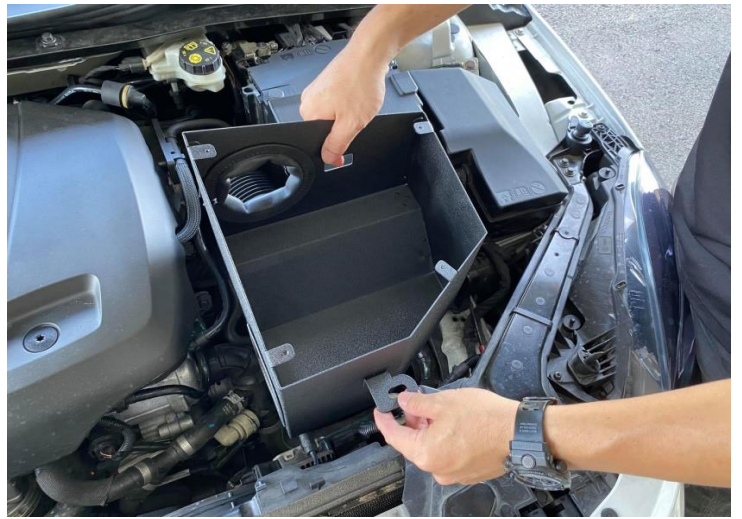
Figure 10: Install the MST heat shield.
