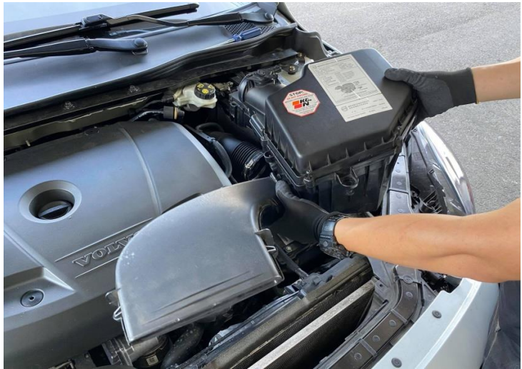
Figure 6: Remove the stock air box.
