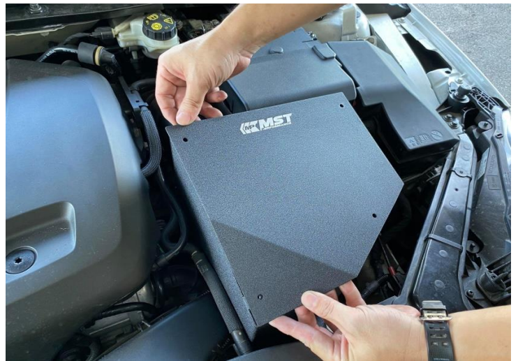
Figure 18: Install the heat shield cover.
