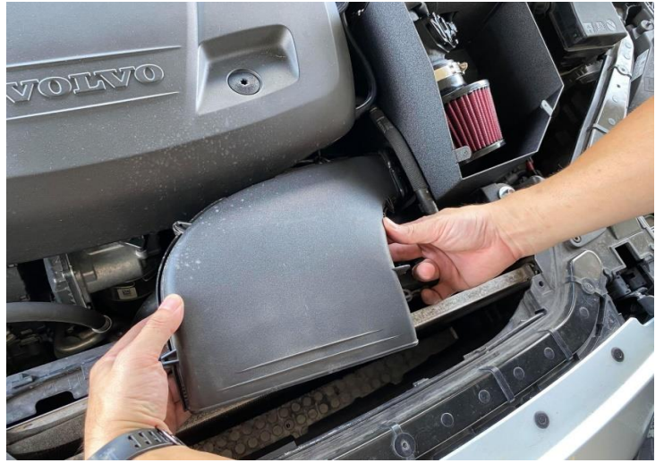
Figure 16: Reinstall the stock air scoop.
