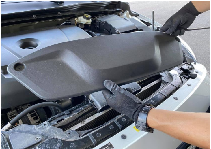
Figure 5: Remove the stock air scoop cover.
