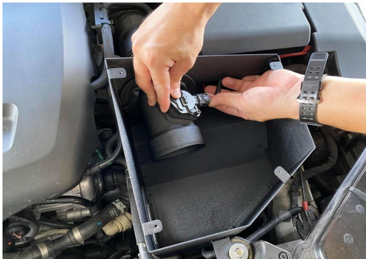
Figure 13: Connect the inlet pipes and tighten the hose clamp.
