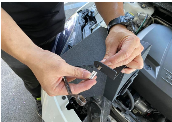
Figure 9: Install the ALU mount.
