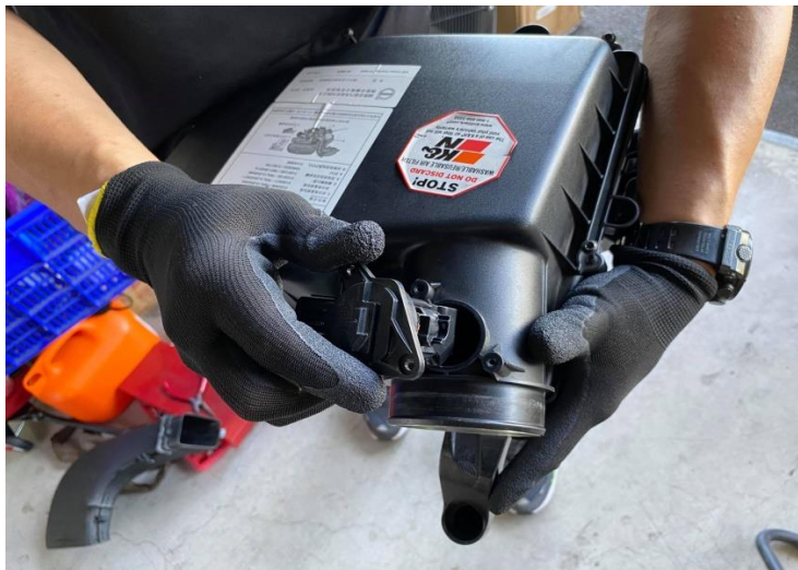
Figure 8: Remove the MAF sensor from the stock air box.
