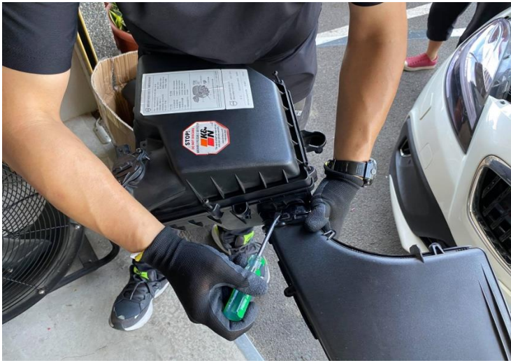
Figure 7: Remove the air scoop from the stock air box.
