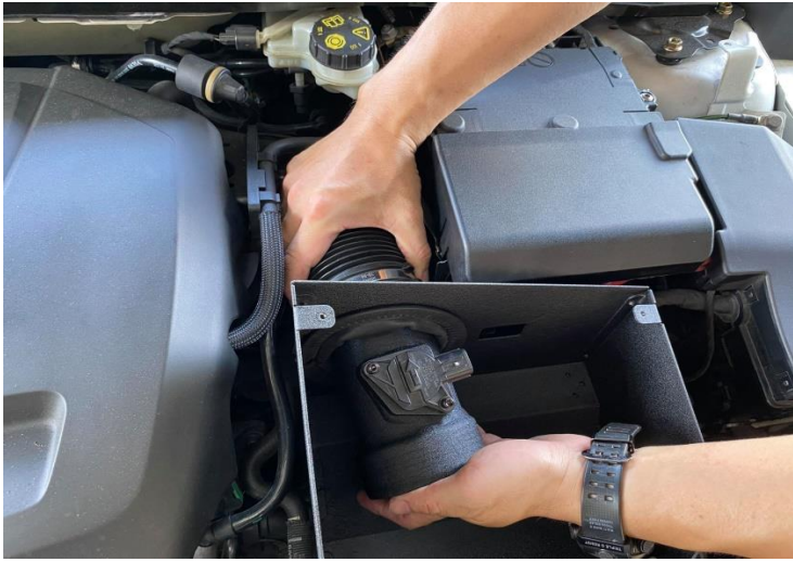
Figure 13: Connect the inlet pipes and tighten the hose clamp.
