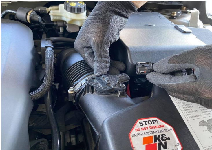
Figure 2: Disconnect the MAF sensor.
