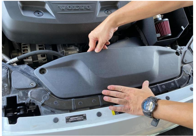
Figure 16: Reinstall the stock air scoop cover.
