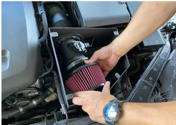
Figure 15: Install the MST filter.
