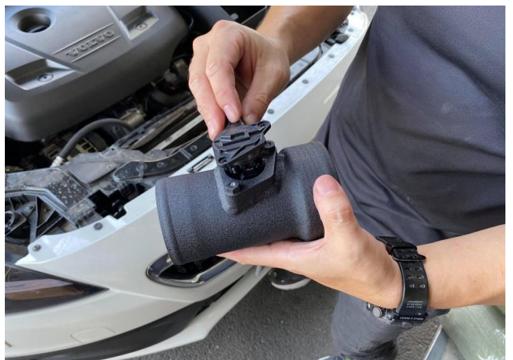
Figure 12: Install the MAF sensor on the MST pipe.
