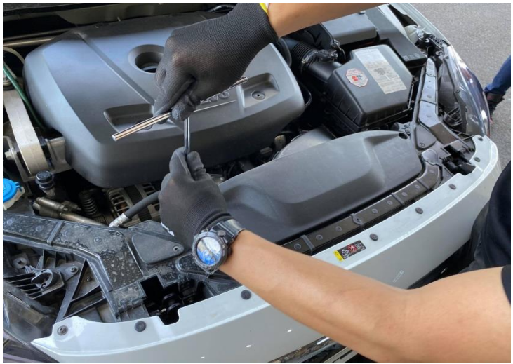
Figure 4: Remove the stock air scoop cover bolts.
