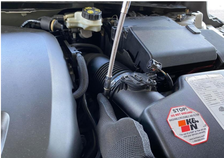
Figure 3: Loosen the hose clamp.
