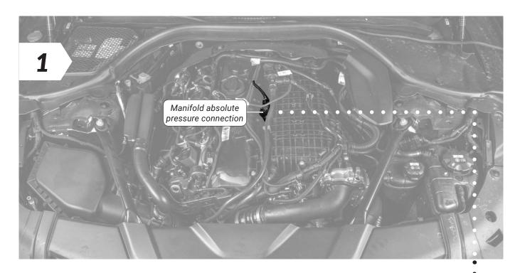
• Once the connection to the turbo boost pressure is complete, it is time to make the connection to the manifold absolute pressure sensor.
