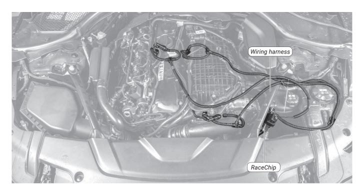
• Before fixing the RaceChip in place in the engine bay, ensure that the wiring harness can also be routed and fixed securely without putting it under excessive tension.
