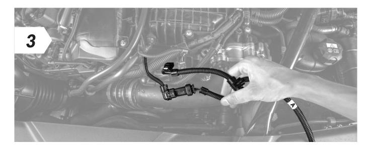
• Now connect the end of the RaceChip wiring harness marked "A" to the disconnected connector and the other end to the sensor.
