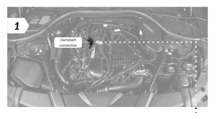
• Once the connection to the manifold absolute pressure is complete, it is time to make the connection to the camshaft sensor.
