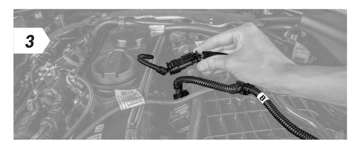
• Now connect the end of the RaceChip wiring harness marked "**B**" to the disconnected connector and the other end to the sensor.
