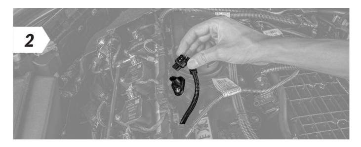
• Disconnect the plug from the camshaft sensor.
