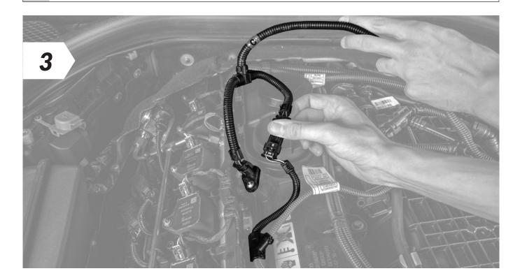
• Now connect the end of the RaceChip wiring harness marked "C" to the disconnected connector and the other end to the sensor.
