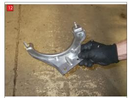
Bolt on transfer box cover plate (item 8) with (item 9) M8x12mm hex head bolts x 7.
