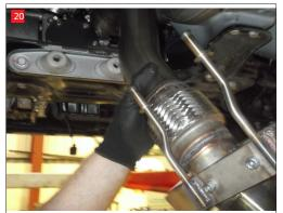
Bolt lower turbo downpipe exhaust mount back on.
