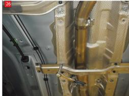
Re-fit lower propshaft cover then tighten up centre racket.
