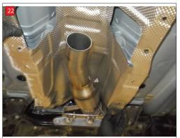
Re-fit v-band clamp (finger tight only, DO NOT FULLY TIGHTEN)
