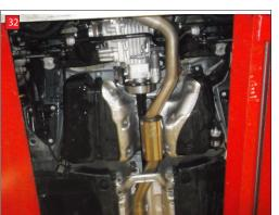
Tighten up v-band on turbo.
