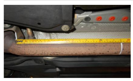
When fitting the Scorpion secondary de-cats the original system requires cutting in a specific place.
