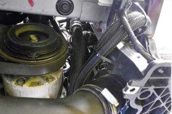
IMPORTANT: Place the cable tie through the loop of the OE loom tie and NOT THE LOOM ITSELF.
