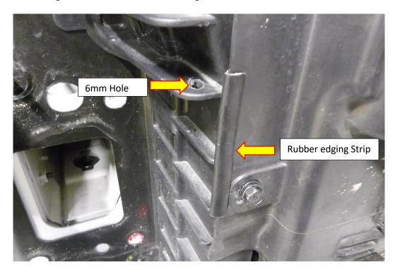
10. Place the crash bar front side down on the floor or work bench, looking at the crash bar with the lower support at the bottom you will see four predrilled holes to the right-hand side. Using a 12.5mm drill enlarge the TWO holes nearer to the centre of the crash bar.
