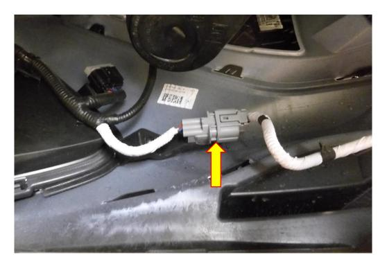
7. Unplug both the temperature sensor and the AAC sensor.
