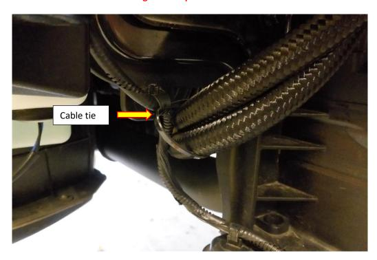
22. Secure the oil lines with a cable tie through the hole made in step 9.
