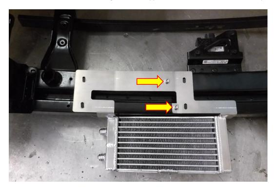
12. Using a white/marker pen mark the centre point of the two holes on the far side of the oil cooler bracket. Now remove the oil cooler from the crash bar and using the 12.5mm drill, produce a hole at both these points and fit the remaining X2 rubber Riv-nuts.
