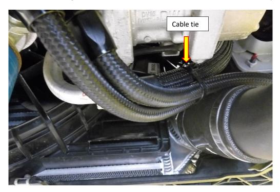
21. Using a 6mm drill make a hole in the fin on the back of the radiator frame next to the intercooler boost pipe, now secure the oil lines using a cable tie inserted through the drilled hole.
