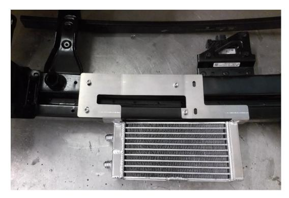
14. Re-fit the crash bar with the attached oil cooler to the vehicle.
