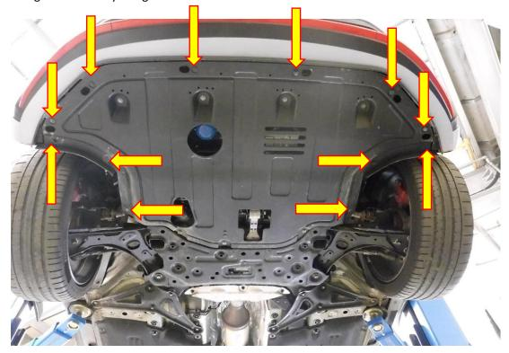
4. Using a 10mm socket and ratchet remove the remaining X7 M6 fasteners and remove the undertray from the vehicle.
