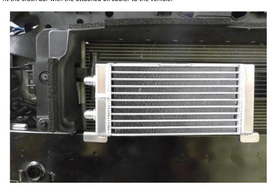
15. Using a marker pen mark out the area in the picture below on the radiator ducting to the left of the oil cooler. With the use of a sharp knife or junior hacksaw cut out the marked section.
