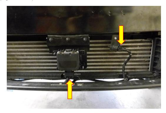
8. Removing the crash bar. Using a 12mm socket and ratchet remove the X8 M10 fasteners X4 each side. Using the 10mm socket and ratchet remove the X4 M6 nuts, X2 each side. The crash bar will now pull away from the vehicle.
