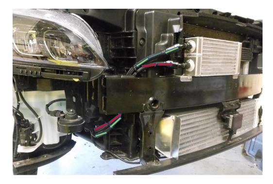
20. Use the supplied cable ties to secure the oil line to the high pressure line, however, do not over tighten it, the lines should still have slight movement, this is the same for all the cable ties used for this procedure.
