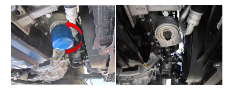
18. Offer up the oil take off plate where the oil filter used to be in the orientation illustrated below, ensuring the rubber O ring side is facing the engine. Using a 26mm extended socket or 26mm spanner secure it in place with the threaded extension supplied. Clean the sealing face for the oil filter, smear a small amount of clean oil on to the oil filter seal, now screw the oil filter onto the threaded extension.
