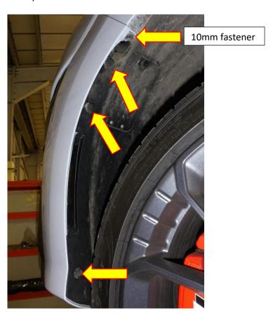
3. With the vehicle raised from the ground, looking up from underneath remove the X12 plastic fasteners attaching the undertray using either a flat blade screwdriver or trim removal tool.
