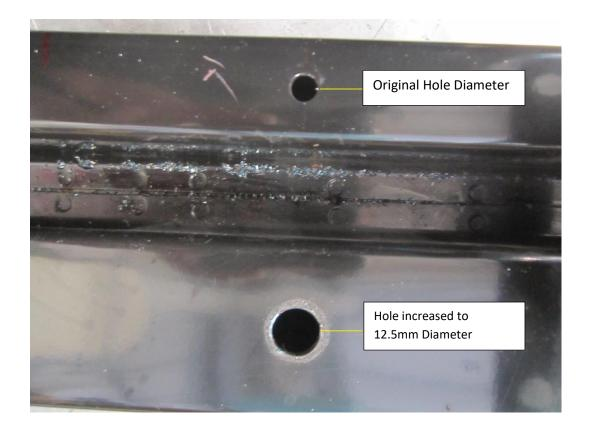
11. Take X2 of the rubber Riv-nuts from the kit and push fit them into the two enlarged holes. Using a 5mm Allen key attach the oil cooler from the kit using X2 of the supplied M6 fasteners as it shows in the picture below.
