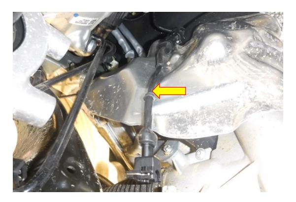
**12**. Route the vacuum hose to the boost solenoid provided and cut the tube to length attaching the vacuum hose to the solenoid as per the diagram pictured below.
