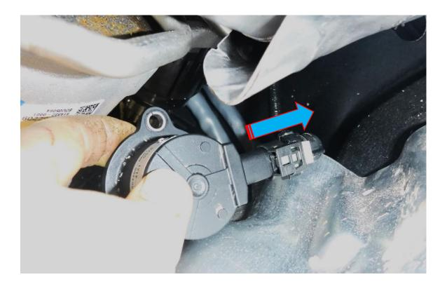
9. Before installing the Forge Motorsport valve, make sure both the large and smaller rubber O-rings are fitted to the base of the valve, they simply push into the relevant grooves.
