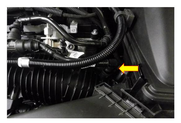
3. Take the supplied split sleeve and slide it over the taper on the pipe (please take note of the orientation).
