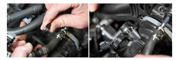
4. Push the supplied adapter over the pipe ensuring the slot is over the split sleeve then secure in place using the supplied horseshoe shape clip.
