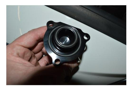
10. Fit the Forge valve to the turbo using the original fasteners and a T30 Torx drive. Please note that the mounting holes are not equally spaced
