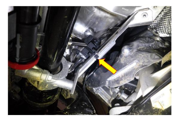
. Connect the DV wiring harness to the solenoid, again make sure to hear it click into position.
