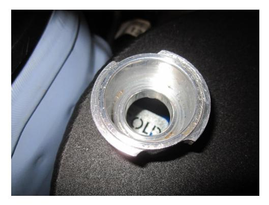
**16.** Take your original coolant cap and screw onto the Forge expansion tank. Once fully tightened place the Forge alloy cap over the OE cap line it up and fix into position with the grub screw.
