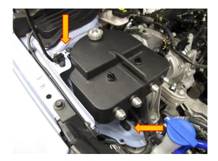
6. If the tank is to be fitted to the **Veloster N** please use the additional bracket and fasteners supplied as pictured below, the nut to the m6 bolt can be tightened from within the wheel arch.
