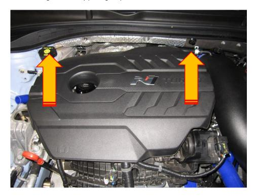
3. Locate the two breather hoses in the engine bay, the first one is at the front of the engine rocker cover and the second one is located at the back of the engine attached to the air intake pipe. To remove them release all four hose clamps in the same way as step one.
