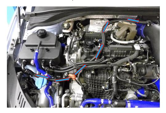
14. The last hose to be installed is another AN-10, run the hose as shown in the picture. As in step 8 the breather end has a push fit machined boss which is secured in place with a M4 fastener. Use 26mm spanners to tighten.
