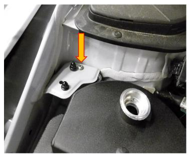
Using a 10mm spanner remove X2 m6 nuts securing the bonnet stay, attach the X2 M6 machined spacers to the M6 studs by screwing them on hand tight. Using a 4mm Allen key attach the bonnet stay to the spacers using the supplied M6x10 fasteners.
