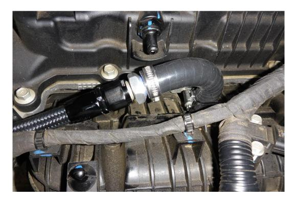
12. Attach the AN-6 fitting of the smaller hose to the catch tank and run the hose to the rocker cover as shown in the picture below. Use a 17mm spanner to tighten the AN-8 fitting and a 7mm socket to tighten the hose clamp on the breather end of the hose.
