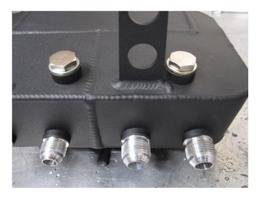
5. Fit the FMCT5 into the same location as the OE expansion tank, fit the lower coolant pipe using the original hose clamp. Secure the tank into place with the fasteners used to hold the OE tank as shown in the picture below. If you find the hose is kinking in the middle cut it's length down slightly.
