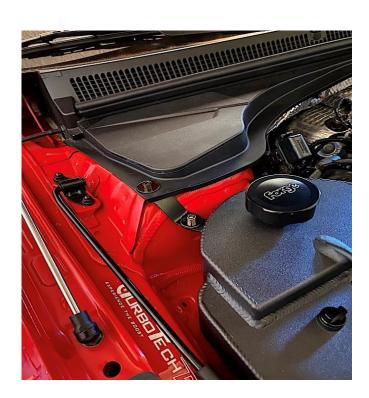
7. If the tank is to be fitted to a **Kona N** you will need to use the S shaped bracket. Using a 4mm Allen key attach the bracket to the catch tank using one of the M6 x 16 button head fasteners and 20mm washer, use the remaining M6x16 button head to attach the bracket to the vehicle.
