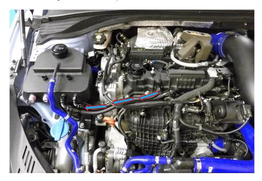
13. Take the longest hose from the kit and run the hose as shown in the picture below. Unclip the wiring loom to the injector behind the oil cap, this will allow you to run the hose underneath it, then re connect the loom. Use a 25mm spanner to tighten the AN-10 fitting and a 7mm socket for the hose clamp at the other end of the hose.
