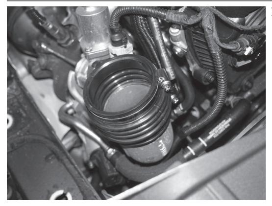
9) Install the APR coupler onto the turbo inlet pipe.
