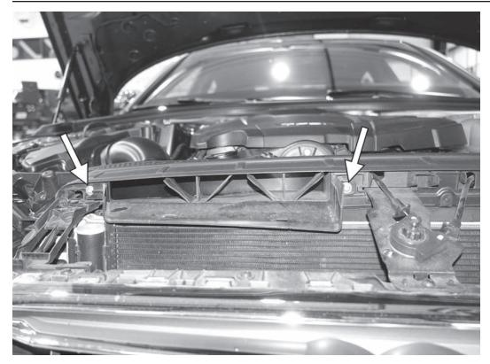
3) Remove the two T25 screws holding the front of the air guide to the radiator support.
