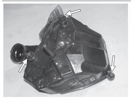
7) Pull off the factory rubber grommets from the bottom of the stock airbox. All three grommets should be on the bottom of the airbox, but may be stuck in the mounting points in the car.
