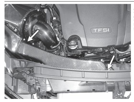
15) Install the APR inlet scoop to the opening on the APR airbox. Push the inlet scoop up against the back of the radiator core support, aligning the threaded mounting holes with the holes on the back of the core support.
