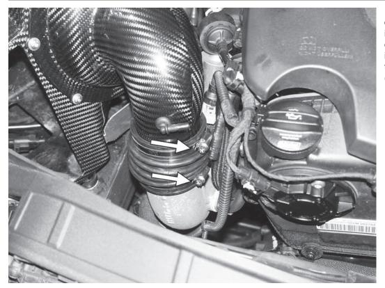
11) Ensure the coupler is correctly over the outlet of the airbox and the inlet of the turbocharger. Position the clamps as show, between the turbo inlet and the side of the engine, and tighten the both clamps to 5.5Nm (48in-lbs).
