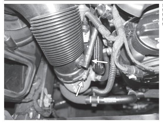
5) Pull off the rubber vacuum line from the plastic 90° fitting on the front of the turbo inlet hose. Loosen the 7mm hose clamp connecting the turbo inlet hose to the turbocharger.
