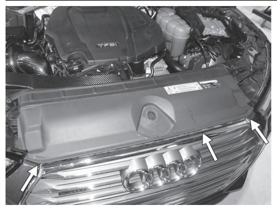
17) Place the back of the hood latch cover into the slot of the radiator support. Then, carefully align the tabs along the front of the hood latch cover and snap them back into their correct positions along the top of the bumper and grill.
