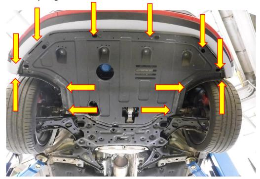
4. Using a 10mm socket and ratchet remove the remaining X7 M6 fasteners attaching the under tray to the vehicle.
