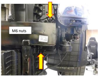
9. Removing the ducting. First unclip the wiring loom that is attached either side of the ducting by using a trim tool or flat blade screwdriver to lever the retaining clip away. Using a 10mm socket and rachet drive remove the 4 fasteners holding the ducting to the car. Once they are removed the ducting can be pulled out, you may have to lever out the two locating pins at the bottom of the ducting when removing.
