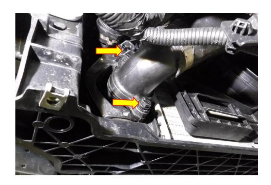
11. Using a 10mm socket and rachet remove the x4 M6 fasteners attaching the OEM intercooler to the vehicle, the intercooler can now be completely removed.
