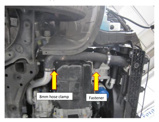
13. Mount the Forge motorsport intercooler in place by angling the left-hand side of the intercooler into position first then the right, once in place use the original M6 fasteners to secure the intercooler to the vehicle.
