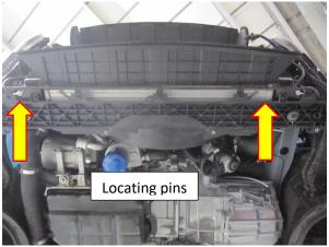
10. To remove the OE intercooler, first undo the hose clamp securing the boost hoses to the intercooler. You will need an 8mm socket and rachet drive or a flat blade screwdriver to loosen them off. Using a 12mm socket and ratchet remove the x2 M8 fasteners attaching the cold side elbow to the intercooler.
