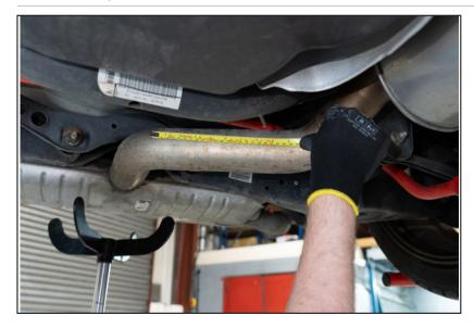
Remove the original system, and measure 110mm from the bend along centre of the pipe
