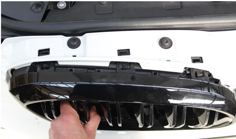
13. Remove the grills – push the tabs in on the top while pulling to release them.
