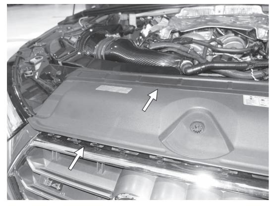
27) Place the back of the hood latch cover into the slot of the radiator support. Then, carefully align the tabs along the front of the hood latch cover and snap them back into their correct positions along the top of the bumper and grill.
