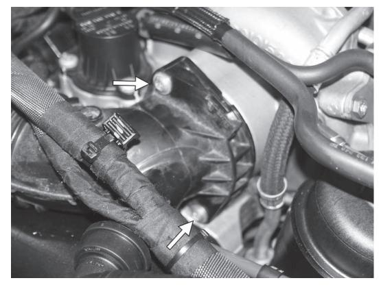
11) Remove the two T30 screws holding the turbo inlet pipe to the front of the turbocharger.
