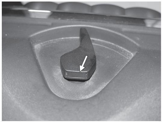
1) Raise the hood and remove the hood latch by pressing in on the small button on the back of the latch, and then lifting the latch up and away from the car. Be sure to not close the hood with the latch removed!
