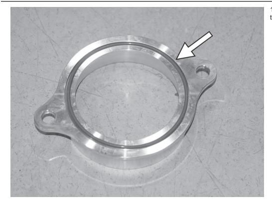
13) Install the supplied O-ring into the billet APR turbo inlet ring.
