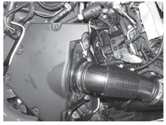
5) Loosen the 7mm hose clamp connecting the turbo inlet hose to the airbox. Separate the turbo inlet hose from the airbox.
