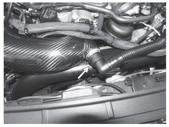
21) Reconnect the PCV hose to the front of the APR turbo inlet pipe by simply pressing the hose onto the port on the front of the inlet pipe.
