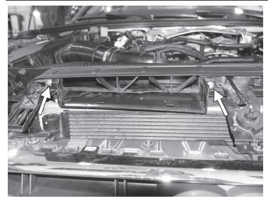
3) Remove the two T25 screws holding the front of the air guide to the radiator support.
