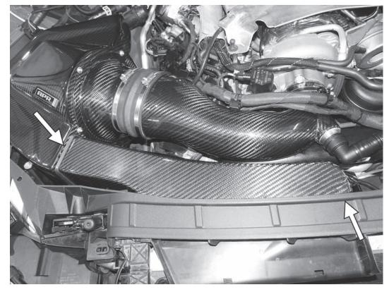
23) Install the APR inlet scoop to the opening on the APR airbox. Push the inlet scoop up against the back of the radiator core support, aligning the threaded mounting holes with the holes on the back of the core support.
