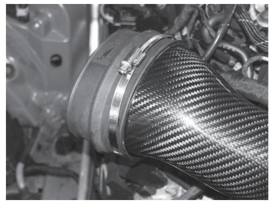
17) On the other end of the APR turbo inlet pipe, loosely install the rubber coupler with one of the hose clamps.
