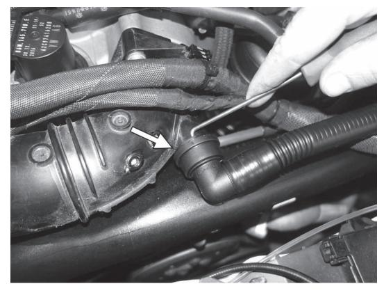
9) Use a 90° pick to loosen the PCV connection on the turbo inlet pipe near the front of the turbocharger.
