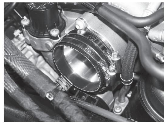
15) Loosely place the supplied silicone coupler with two hose clamps over the APR turbo inlet ring as shown.
