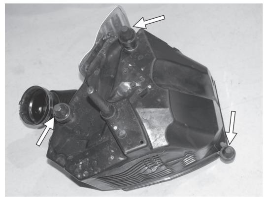
7) Pull off the factory rubber grommets from the bottom of the stock airbox. All three grommets should be on the bottom of the airbox, but may be stuck in the mounting points in the car.
