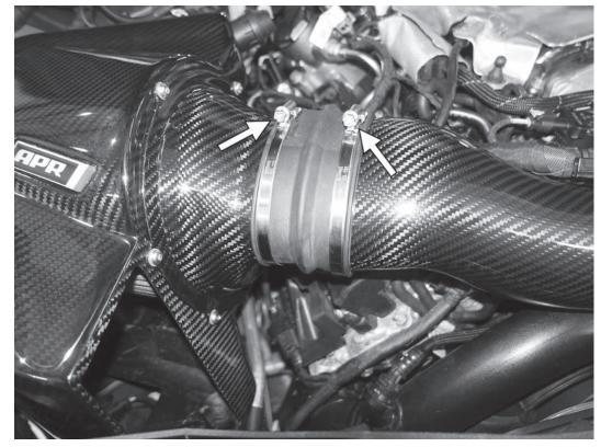
19) With the second 7mm clamp, slide the coupler between the APR airbox and the APR turbo inlet pipe. Make sure the coupler is even on both sides of the connection, and then tighten the clamps to tighten them to 5in-lb (0.6Nm). Do not overtorque the clamps, as you can crush the carbon fiber intake. This torque spec is very low, but the intake will be secure.
