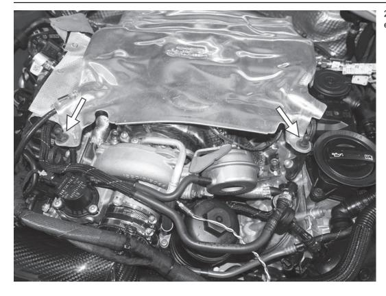
25) Remove the two front 13mm engine cover mounting posts.
