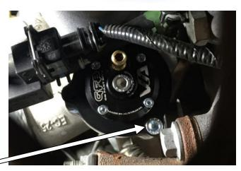
Position the solenoid mounting bracket over the VTA, then insert the remaining two longer mounting screws into the bracket and VTA. All three screws can now be tightened.
