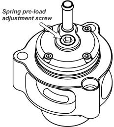
Adjusting the spring pre-load changes how easily the valve vents when the ECU triggers. The best throttle response is typically found when the spring is set as firm as possible without causing compressor surge (turbo fluttering) when the throttle is closed on a high boost/high RPM gearshift.
