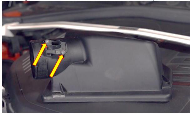
7. Using a 3mm allen key and suitable drive, attach the MAF sensor to FMINDK55 with the supplied bolts.
