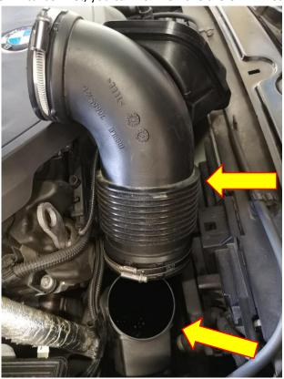
5. Using your hand release the four metal clamps that hold the upper airbox in place and remove it from the vehicle by pulling it up vertically.
