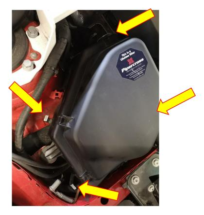
6. Using a T20 and suitable drive, remove the MAF sensor from the OEM upper airbox.
