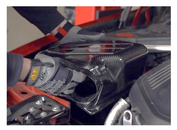
10. Place the supplied hose clamps around either end of the inlet hose and attach that longer end of the hose to the OEM turbo inlet. As you have the airbox in position you can use that to line up the other opening and attach it to FMINDK55. FMINDK55 was not latched down so that it does not impede the installation of the inlet hose.
