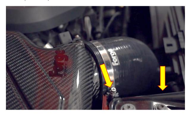
13. Reattach the MAF loom by clicking it back into the MAF sensor.
