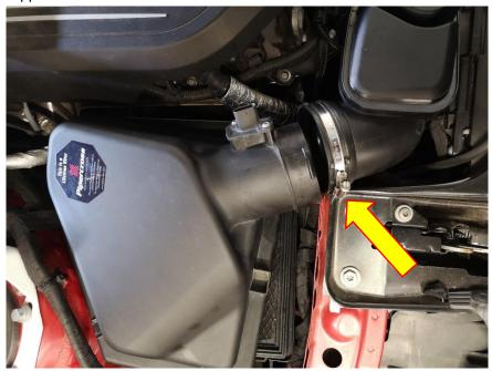
4. Using a 7mm socket and suitable drive undo the bottom of the OEM inlet hose where it attaches to the OEM turbo inlet, you can now remove the OEM inlet hose.
