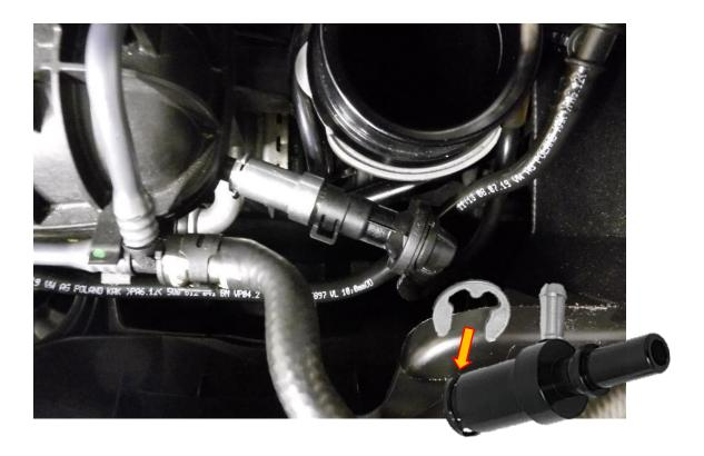
11. Fit the Forge Motorsport silicone hose into place and secure it with the two hose clamps supplied, 70-90mm clamp on the larger end of the hose and 40-60mm on the smaller end. Use a 7mm socket and rachet to tighten the clamps.
