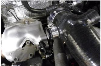
13. On the intake hose of FMINDK35 you will see the extra spout, use the supplied 20mm hose joiner and secure it in place with the 16-27 hose clamp.
