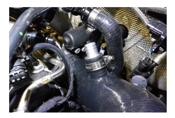
14. Take the silicone hose marked #2006 and fit the smaller end to the hose joiner fitted in the previous step and secure with the supplied 16-27 hose clamp. Fit the Forge valve in the same orientation as shown in the picture below, secure in place with the supplied 20-32 hose clamps.
