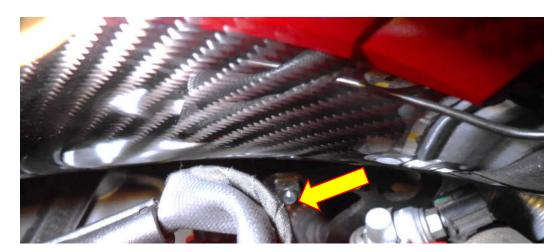
23. Reinstall the OEM cold air feed duct with the OEM Torx screws
