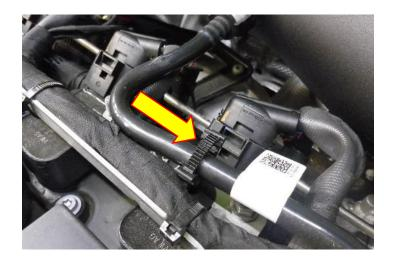
6. Squeeze the sides of the norma clip so that the PCV pipe can be disconnected from the inlet pipe.
