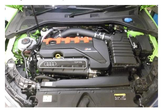
2. Using a T25 and suitable drive remove the x2 Torx screws that hold the cold air feed duct to the vehicle.
