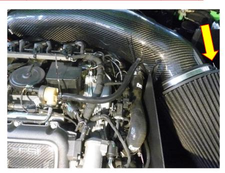
**21.** Using a 7mm socket and suitable ratchet tighten the hose clamp on the turbo inlet end.
