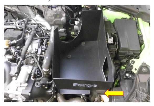
**18**. Install the carbon fibre section of FMINDK47, by sliding the adapter into the turbo inlet hose and then slowly lowering it down until the bracket is lined up with the bolt
