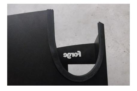
17. Install the heat shield as shown below. There is a tab at the front of the heatshield which can be used to connect the gearbox breather.
