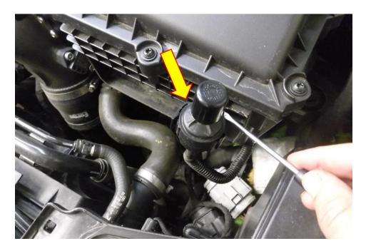
**9.** A. FOR NON-OEM TURBO INLET. Using a 7mm socket and suitable drive loosen the hose clamp which connects FMINLH9 to FMINLH8.
