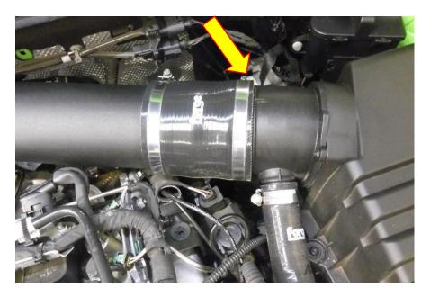
B. FOR OEM. Using a 7mm socket and suitable drive loosen the hose clamp connecting the OEM hose to the OEM airbox. Pull the hose off the OEM airbox.
