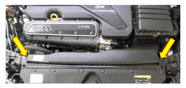
3. Push the cold air feed duct towards the airbox and then pull vertically and towards you to remove it from the vehicle.
