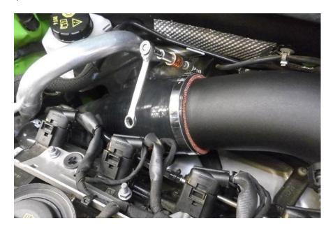
B. FOR OEM TURBO INLET. Using a hose clamp removal tool or pliers, disconnect the sprung clamp that holds the OEM inlet hose to the OEM metal turbo inlet.
