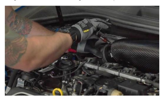
22. Using a 5mm torx bit and suitable drive, tighten the M6 fastener (making sure to include the M6 spring washer and penny washer)
