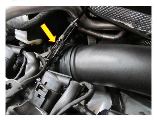
**10**. A. FOR NON-OEM. Using a 7mm socket and suitable drive loosen the hose clamp connecting the silicone hose to the OEM airbox. Pull the hose off the OEM airbox.
