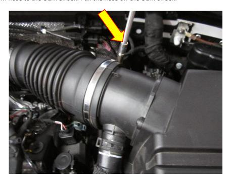
**11.** Using either a 7mm socket and suitable drive or a hose clamp removal tool (depending on the hose), disconnect the diverter valve recirculation hose from the OEM airbox.
