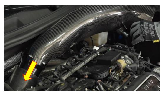
19. Push the diverter valve recirculation hose over the lower of the two protruding pipes from FMINDK47 and tighten the associated hose clamp with a 7mm socket and suitable drive or a hose clamp removal tool. Push the supplied hose over the pipes from the plastic PCV and FMINDK47 as shown in the image below (trim if necessary). Clamp to pipes using the supplied cable ties and trim with flush faced cutters.
