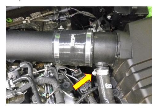
12. Using a T25 bit and suitable drive, reach your hand between the inlet pipe and the firewall to undo the fastener holding the inlet pipe in position. You can now remove the OEM/ Forge Motorsport inlet pipe from the engine bay.
