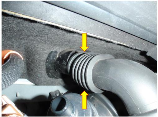
5. You can now remove the lower 10mm bolt holding the noise generator to the side of the engine using a ratchet spanner from the front or  $\frac{1}{4}$ " drive ratchet from the back, and remove the noise generator from the car.
