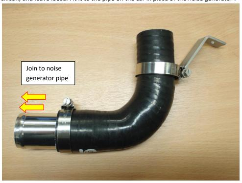
10. Fit the valve to the end of the pipe and tighten the jubilee clip whilst positioning the bracket under the hole in the firewall. Using a 10mm socket and spanner tighten the M6 fastener and penny washer on the top of the bracket, and the plain washer and Nyloc nut on the bottom to secure the bracket. Connect the vacuum hose between the top of the valve and the tee piece in step 6 use the supplied cable ties to secure the vac hose and use side cutters to cut the excess.
