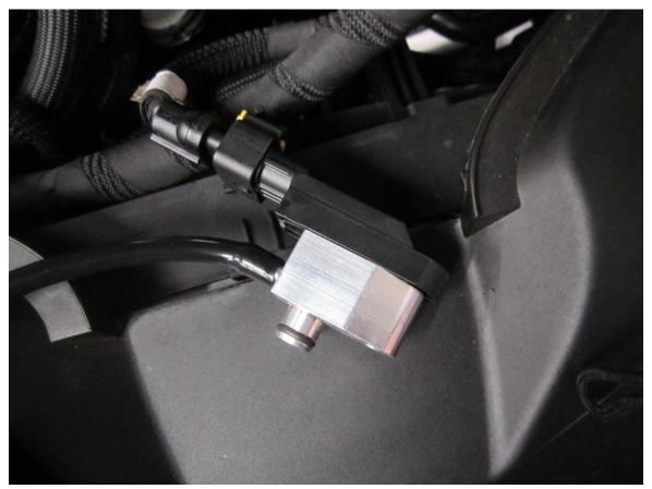
6. Refit the map sensor and boost take off with the m6x35mm provided then route the vacuum tube to your desired location.
