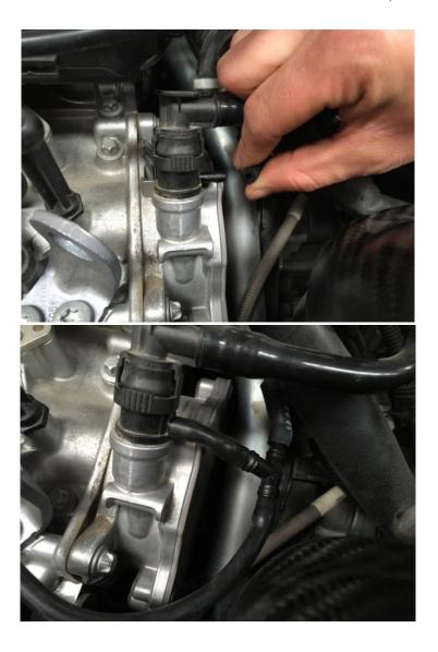
6. Mount the solenoid close to the BOV – in this instance we have used one of the bolts of the BOV, and plumb it up as shown in the diagram below, by cutting the vacuum hose to length.
