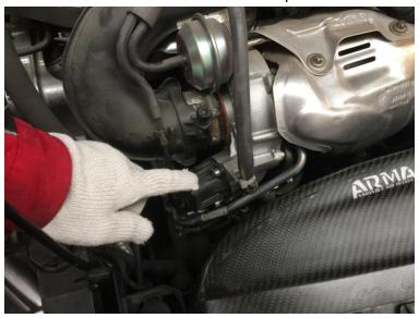
3. Remove the valve by disconnecting the plug and removing the 3 bolts.
