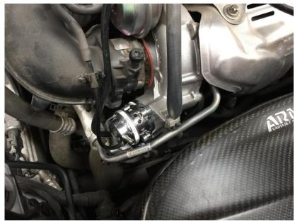
5. Locate the vacuum pump on the right hand end of the engine (when viewed from the front), and remove the small bore vacuum hose from the side of the outlet. Use the supplied tee piece as shown below to connect to the pump outlet with a short length of vaccum hose, and then connect the coil of vacuum hose to one other side and run it over to the BOV neatly.
