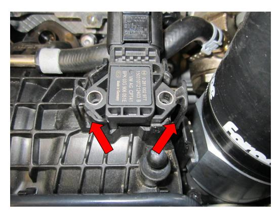
2. The boost tap block must now be placed in position on the manifold, make sure the cork gasket is placed beneath the boost tap block then push down again until you feel it click into position
