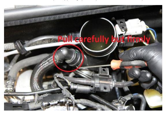
Transfer o-ring from factory part to CTS inlet. Install CTS inlet, secure by turning counterclock wise (towards front of vehicle) and tighten the T30 screw.
