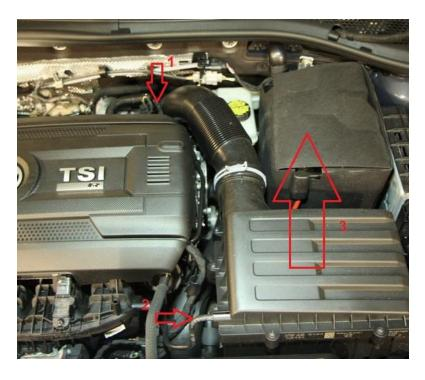
Step 4: Remove two 7mm clamps on the turbo outlet.
