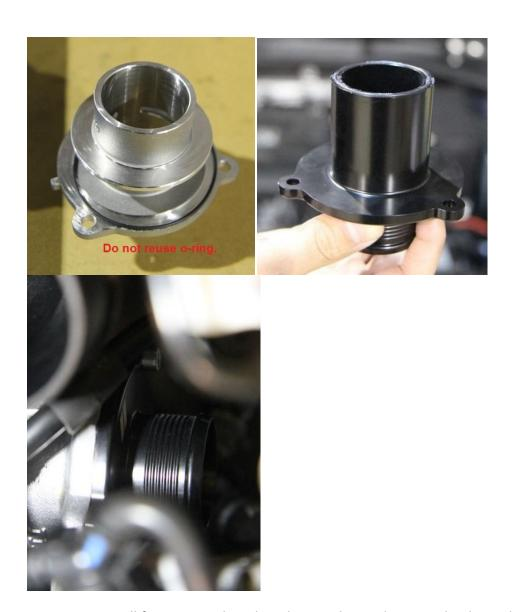
Step 10: Reinstall factory coupler, align the coupler as shown and tighten clamps. Reinstall turbo outlet pipe, DSG breather (if equipped) and air intake.
