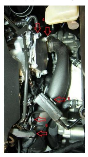
Step 7: Remove the rubber turbo outlet pipe coupler. Move the outlet pipe out of the way (having a friend help is good).
