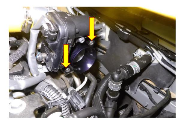
6. Fit the new FMTIA4 hose in place as shown in the picture below, secure the hose using a 7mm socket and ratchet and the supplied 60-80 hose clamps.
