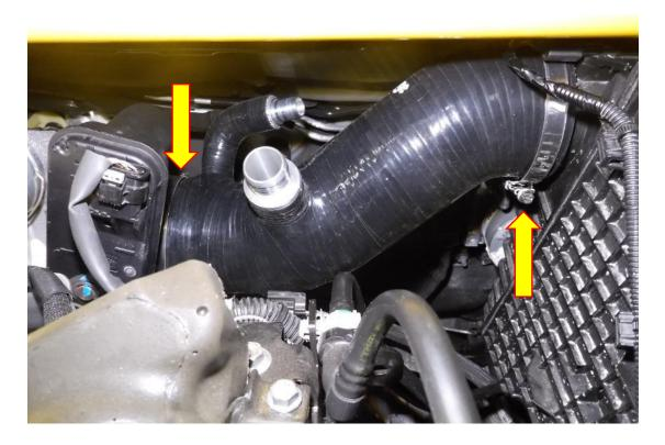
7. Re-fit the oil breather hose and DV hose to the billet adaptors on the FMTIA4 hose. That is the installation of FMTIA4 complete, take the vehicle for a test drive and enjoy your new Forge Product.
