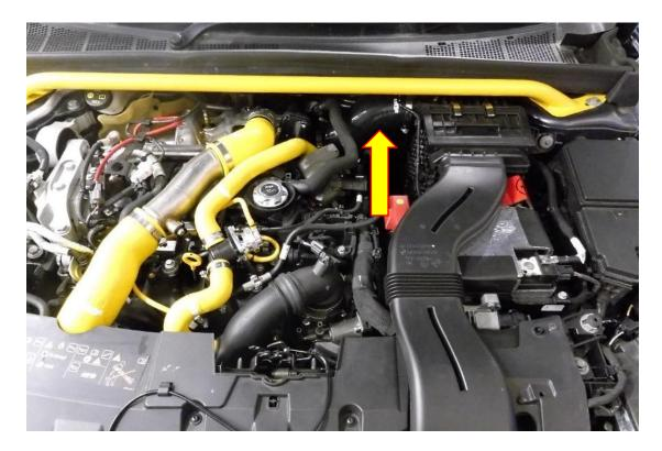
2. Using your hose clamp removal tool or 7mm socket and ratchet loosen both hose clamps attaching the OE turbo inlet hose.
