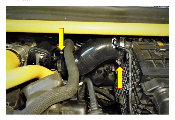
3. Using a hose removal tool remove the oil breather hose and the DV hose from the OR inlet elbow. With both hoses removed you will now be able to remove the turbo inlet hose from the vehicle.
