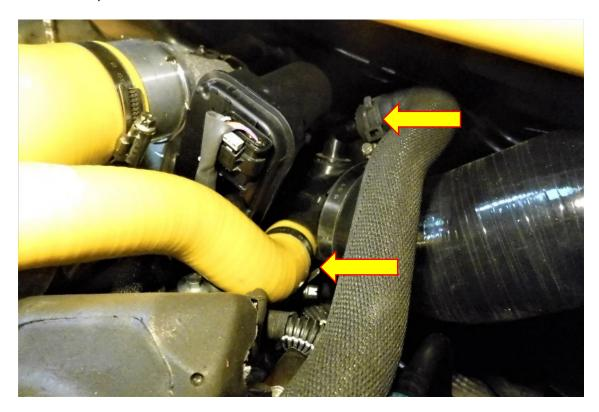
4. Using a 13mm socket and ratchet remove the two M8 fasteners attaching the OE turbo elbow to the turbo.
