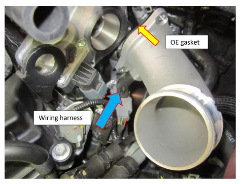
4. Take the Forge Motorsport machined turbo adaptor and offer it up to the OE gasket as shown in the pictures below.
