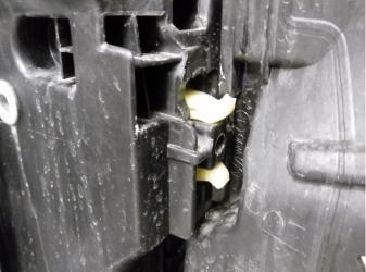
29. Using a flat blade screwdriver or trim tool, push both retaining clips down to separate the radiator from the intercooler. Once parted lift the radiator upwards from the intercooler to completely remove the radiator from the intercooler.
