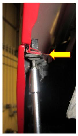
9. Using a T25 Torx and drive remove the x7 M5 fasteners attaching the bottom of the bumper.
