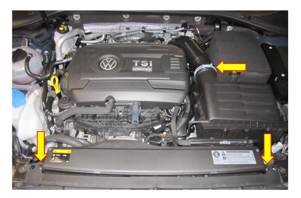
4. Unclip the coolant hose from the front of the airbox lid. Disconnect the vacuum hose attached to the front left of the airbox.
