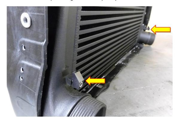
**34**. Fit the radiator to the intercooler, make sure the lower locating pegs of the radiator are seated inside the clamps, push the upper retaining clips into position to secure the radiator. Using a 6mm Allen tighten the clamp.
