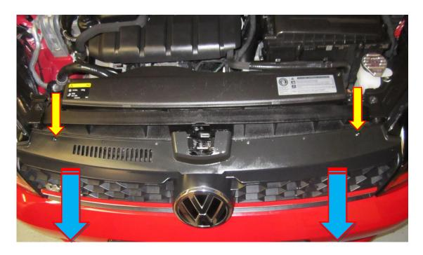
3. Using a T25 Torx and drive remove the x2 M5 fasteners that hold on the airbox duct and use a hose clamp removal tool to loosen the inlet hose from the air box.
