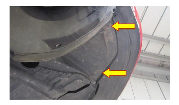
10. Using a T25 torx and drive remove the x8 M5 fasteners attaching the undertray to the vehicle.
