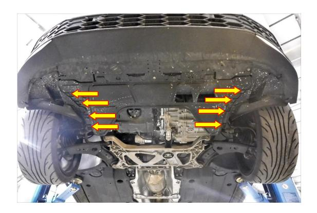
11. Pull sharply on the sides of the bumper to release them from the vehicle. You will now be able to release the bumper from the vehicle but not fully, but enough to allow access to unplug the fog lights and parking sensor connector. Also find a suitable container to catch the washer fluid as the light washers also need to be disconnected.
