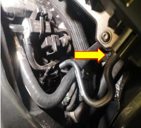
5. The airbox is located by rubber grommets on three pins. Rock the airbox left to right while pulling in an upwards motion to remove it. You can now remove the front air ducting highlighted with the yellow arrow.
