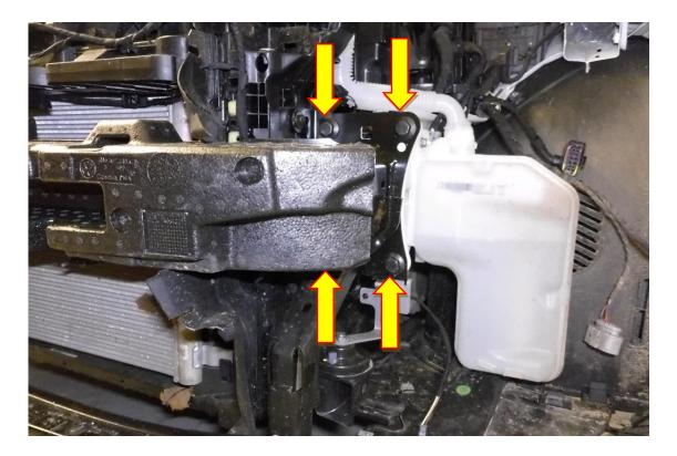
25. Using a 10mm socket and ratchet remove the X2 M6 nuts that hold the slam panel to the crash bar .
