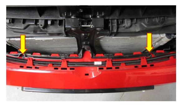
7. Using a T25 Torx and drive remove the x4 M5 fastener on both sides of the wheel arch liners.
