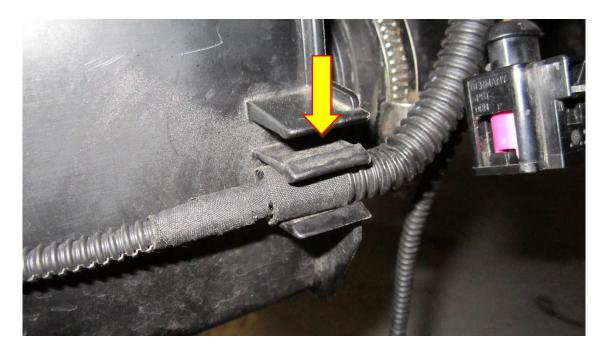
20. Disconnect the loom from the temperature sensor clipped to the lower of the crash bar. If your vehicle is equipped with ACC disconnect this also, but be careful ton to bend the bracket attaching it to the crash bar.
