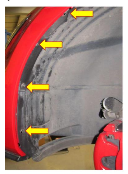
8. Peel back the top of the arch liner to reveal the M5 fastener on each side and use a T25 Torx and drive to remove them. Now using a 10mm socket and rachet remove the plastic nuts attaching the plastic
