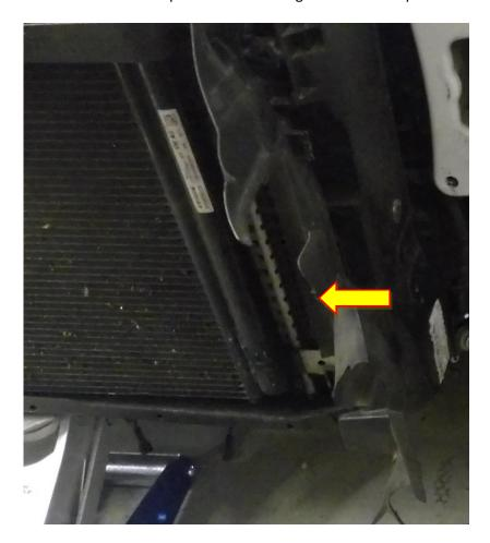
**27.** Push in the locking tabs securing the air conditioning condenser, lift the unit upwards to release it from the radiator pack.
