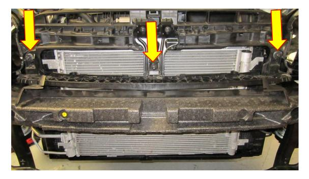
17. Using a muiltispline 12 socket remove the horn brackets and disconnect the loom on either side of the vehicle
