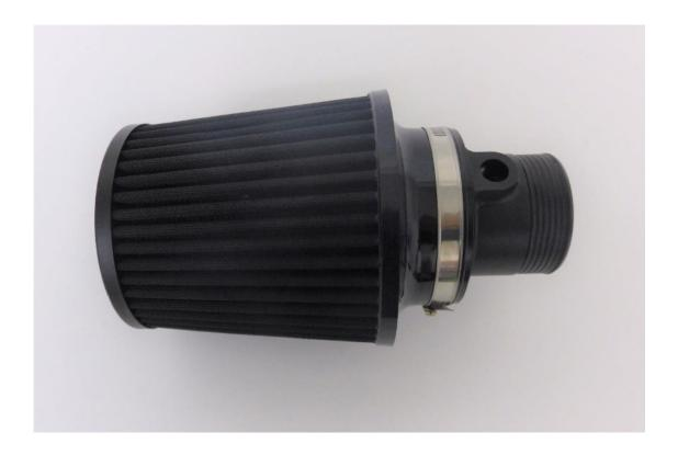
6. Attach the MAF tube and air filter to the intake hose and re-fit the MAF sensor.
