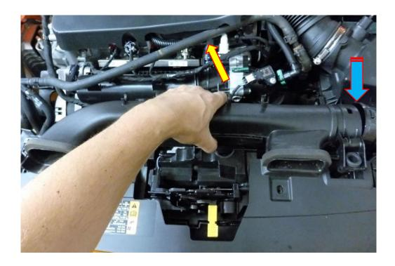
3. Twist the MAF sensor anti clockwise and remove it from the airbox, there is enough length in the cable to place it on the battery for now. Using a 7mm socket and ratchet loosen the hose clamp enough so the hose can be removed. Pull the airbox Sharpley in an upwards motion and remove from engine bay.
