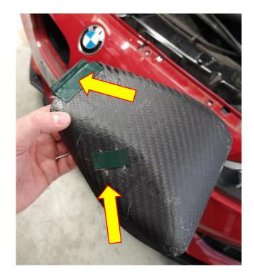
12. Feed 2 of the supplied cable ties through FMINLD2 as shown below. At this point it is worth lining up FMINLD2 on the vehicle to see how it fits up before you remove the backing from the double-sided tape. You want the long straight edge to be vertical, so it lines up with the slats in the kidney grill.
