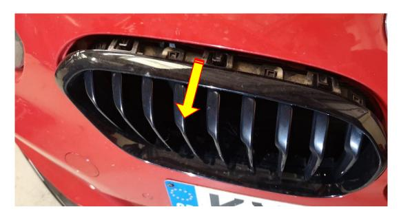
7. Slide your hand in between the final few slats on either the left or right side of the kidney grill and reach for the singular tab on the side. Depress the centre of the tab in the same way as the previous step, and then use your other hand to gently pull the kidney grill surround towards you to release. Repeat this for the other side of the same kidney grill.
