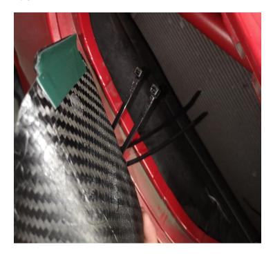
13. Remove the backing off the double-sided tape. Line up FMINLD2 inside the opening, with the cable ties going around the support bar. Hook the end of FMINLD2 around the corner of the opening and push firmly for 30 seconds to ensure good adhesion.
