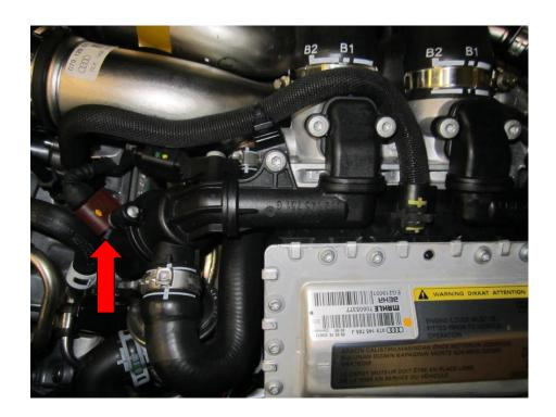
4.Using a T30 Torx Driver, remove the 3 fasteners from each OEM valve, then remove them from their housing.
