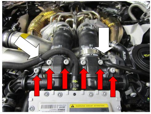
3. Disconnect the wiring loom to each OEM valve, these are both brown plugs.
