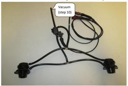
15. Now connect the Forge Motorsport wiring loom to the solenoid and then to your OEM wiring loom.
