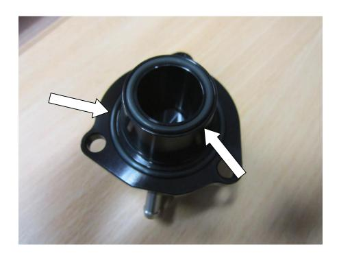
6. You can now fasten the Forge Motorsport valves to the housings again using your T30 Torx driver. Please note the orientation of the valve.
