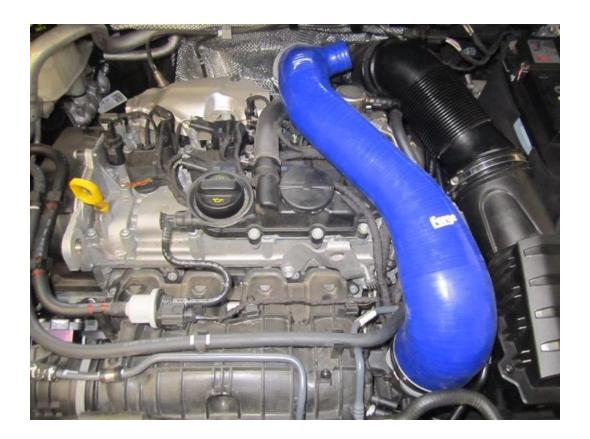
11. Fit the Forge dump valve to hose and secure into place with the 20-32mm hose clamp.
