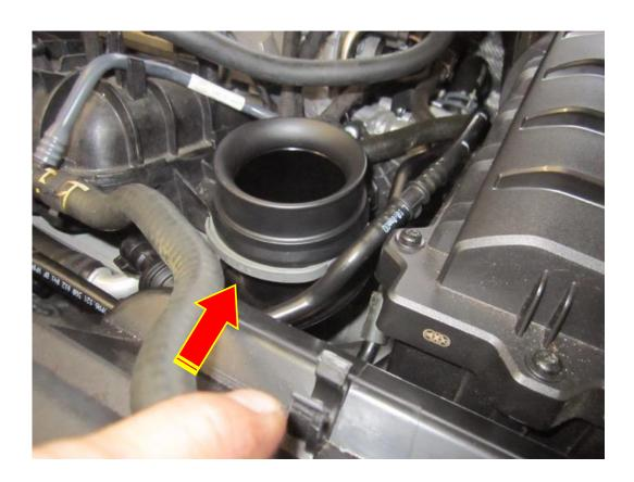
7. Fit the supplied O ring into the machined slot of the smaller two-piece Forge coupler as shown in the picture below.
