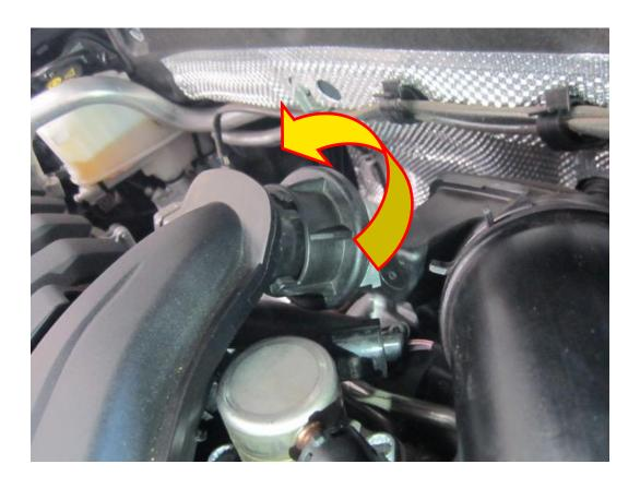
4. With the use of a flat blade screwdriver or trim tool, release the plastic retaining clip which holds the other end of the boost inlet pipe. The boost pipe will now be free at both ends and will pull away from the engine bay.
