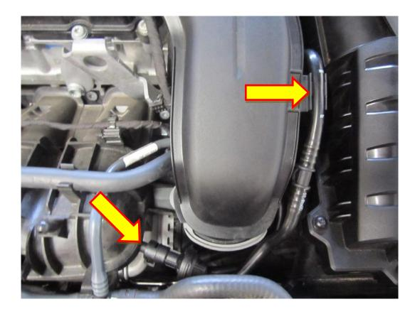
3. At the end of the boost inlet pipe nearest the back of the engine, turn the twist fit coupler anti clockwise to unlock it.
