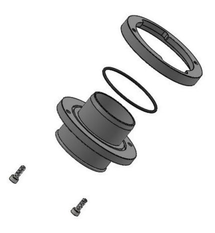
9. Place the two-piece Forge Motorsport billet coupler onto the turbo outlet by locating the two key way cut outs on the back of the coupler over the tabs on the turbo out-let. Once in place twist either clockwise or anti clockwise as far as possible then tighten the two M4 fasteners with an Allen key.
