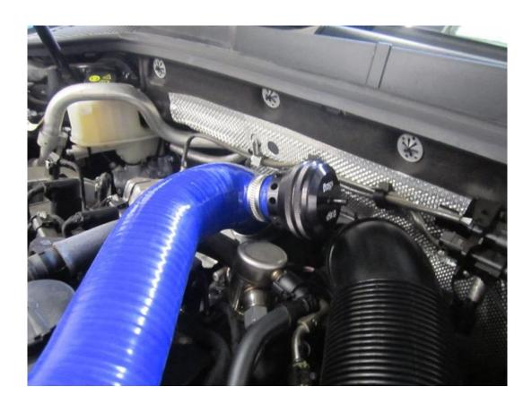
12. Push the Forge vacuum T over the vacuum port on the inlet manifold, secure it with the E-clip provided and reconnect the OEM vacuum hose (removed in Step 2.) to the other side of the Forge vacuum T.
