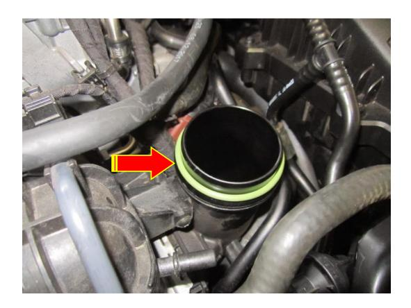
6. Fit the larger single piece Forge Motorsport billet coupler over the charge cooler in-let pipe and secure in place with the OE plastic retaining clip.
