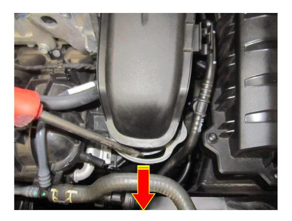
5. Remove the factory O-ring from the coupler on the OE boost inlet pipe and place it on the charge cooler inlet pipe.
