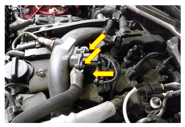
4. Place FMSP3 in position where the OE dump valve was located, then fit the valve on top of the Forge sandwich plate and using a pozi drive screwdriver secure them using supplied fasteners.
