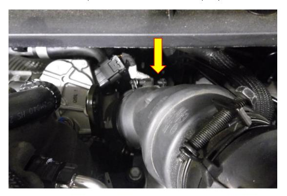
4. Using a flat bladed screwdriver prise the X2 plastic retaining clips open and remove them from the air duct.
