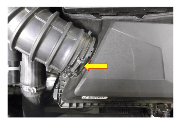
3. Again, using a 10mm socket and ratchet loosen the hose clamp and remove the opposite end of the inlet hose attached to the turbo adaptor. You can now remove the hose completely.
