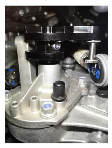
14. Using either a 10mm spanner or socket and suitable drive tighten the hex head bolt.
