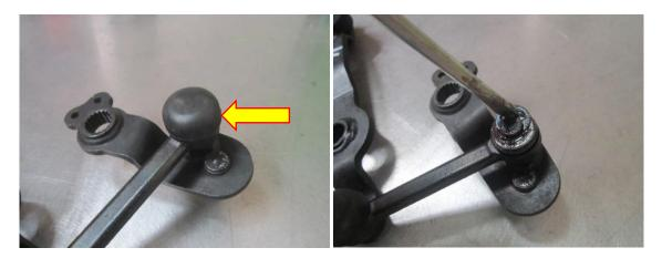
8. At this point you will need to set up your new Forge Motorsport short shift linkage. Assemble the link as shown in the diagram below using a 13mm spanner or socket and rachet to tighten the cable pins in place, the pins have two flat edges to locate it securely in the slot. These pins are the adjustment for the shift length, to make the shift shorter move the pin closer to the toothed location hole. Please Note:
