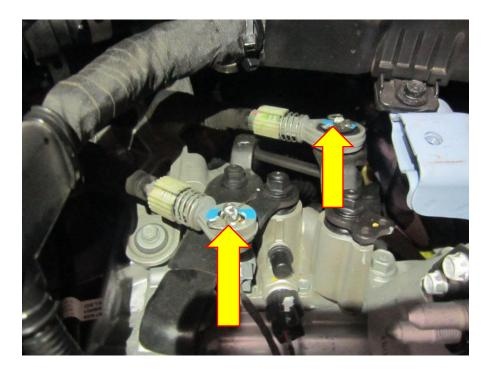
6. There are three 14mm fasteners that hold the linkage to the gearbox. Remove these with a 14mm socket and rachet, with these removed the linkage will lift off with gentle persuasion.
