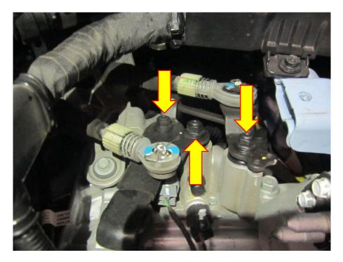
7. With the OE gear linkage removed from the vehicle you will now be able to split the back and forth part of the linkage. Remove the rubber dust cover shown in the picture, with that removed you will see a circlip holding the linkage together. With the use of a flat blade screw driver prise the circlip out of its mounting, this will then allow you to remove the back and forth part of the linkage
