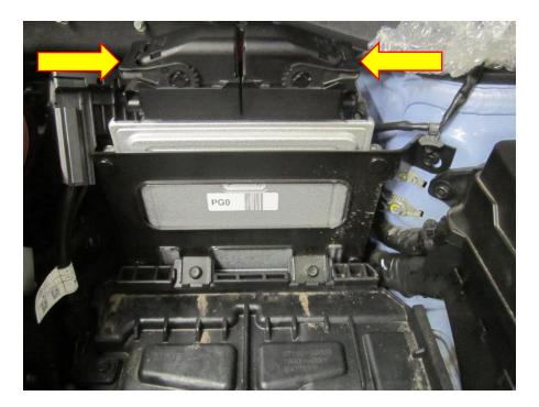
3. Once unplugged you can now remove the three 10mm fasteners that hold the ECU in position, two at the bottom and one at the top right. Use some long nose plyers to remove the plastic fastener that is holding the negative battery cable to the ECU bracket.
