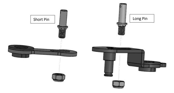
9. You can now fit the Forge back and forth linkage to the OE part as illustrated below, this is the reverse of step 7.
