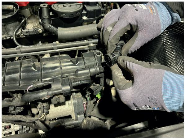
3. Now remove the two ignition coils of the third and fourth cylinders.
